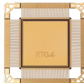
RTG4™ Radiation-Tolerant FPGA
