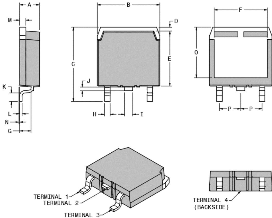
The following table shows the TO-268 dimensions and should be used in conjunction with the package outline drawing.
