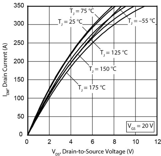
**Figure 2 • Drain Current vs. Drain-to-Source Voltage**
