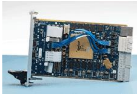
RTG4 PX1e® board used to validate the SpaceFibre router
