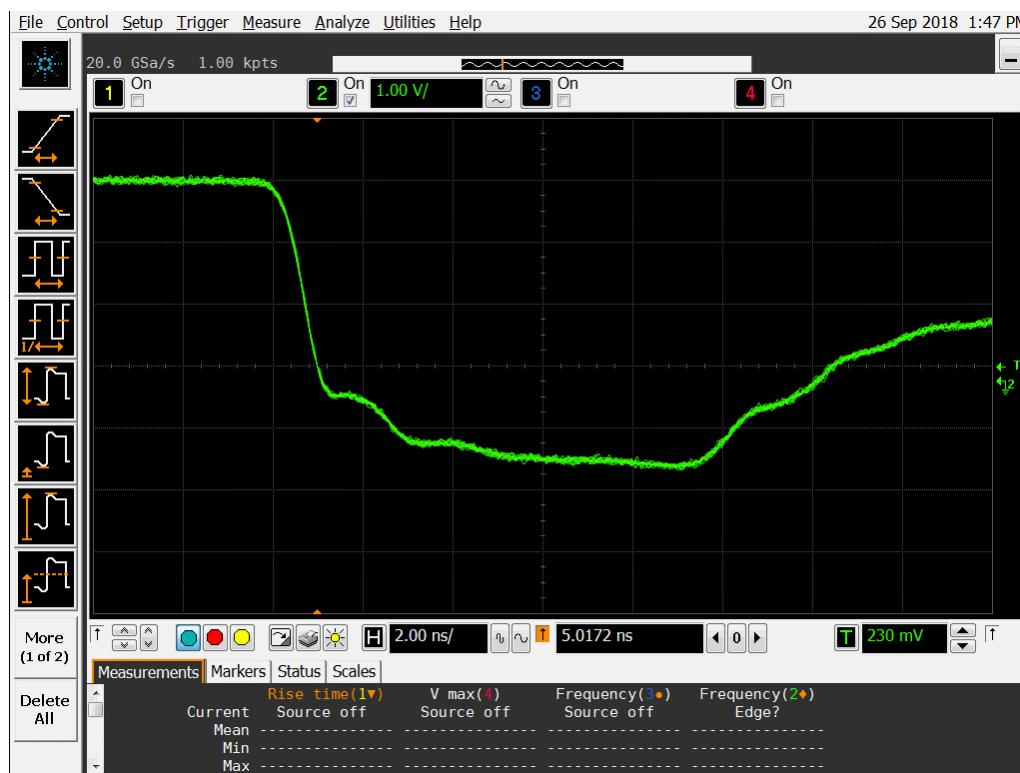
**Figure 16a DUT 7128 Pre-Irradiation Falling Edge.**
