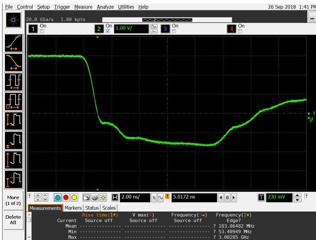
**Figure 19a DUT 7118 Pre-Irradiation Falling Edge.**
