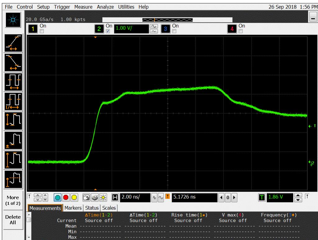
Figure 9a DUT 7146 Pre-irradiation Rising Edge.
