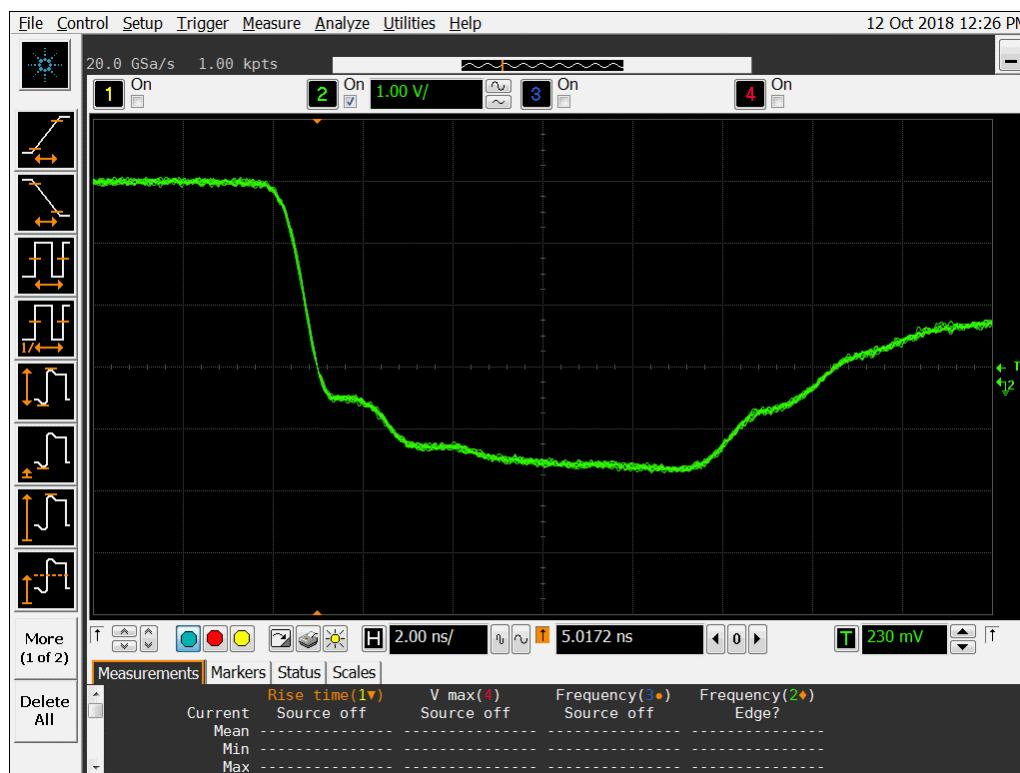
**Figure 18b DUT 7111 Post-Annealing Falling Edge.**
