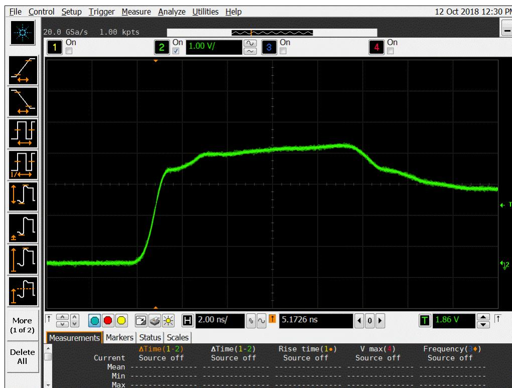
**Figure 10b DUT 7128 Post-Annealing Rising Edge.**
