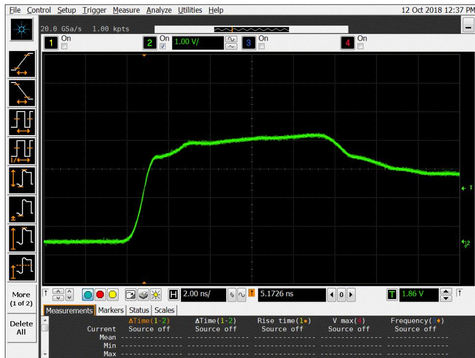
Figure 8b DUT 7141 Post-Annealing Rising Edge.
