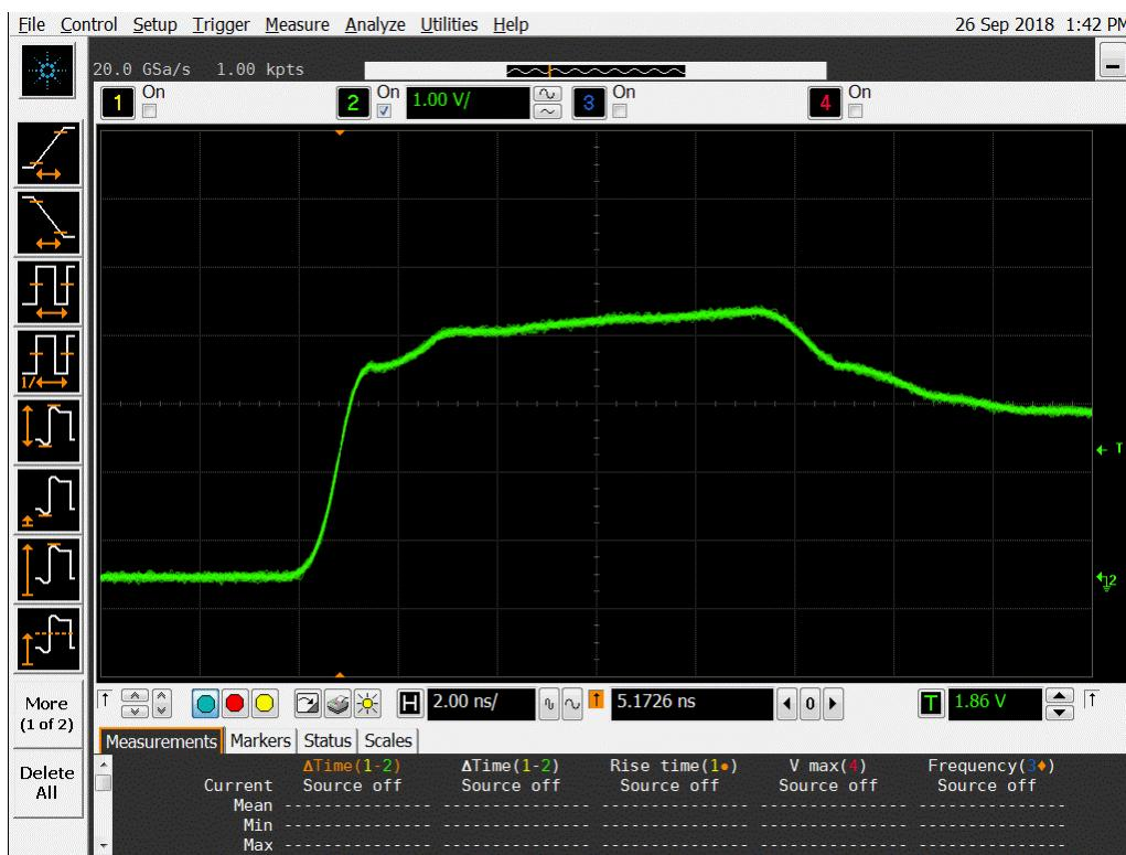
**Figure 13a DUT 7118 Pre-Irradiation Rising Edge.**
