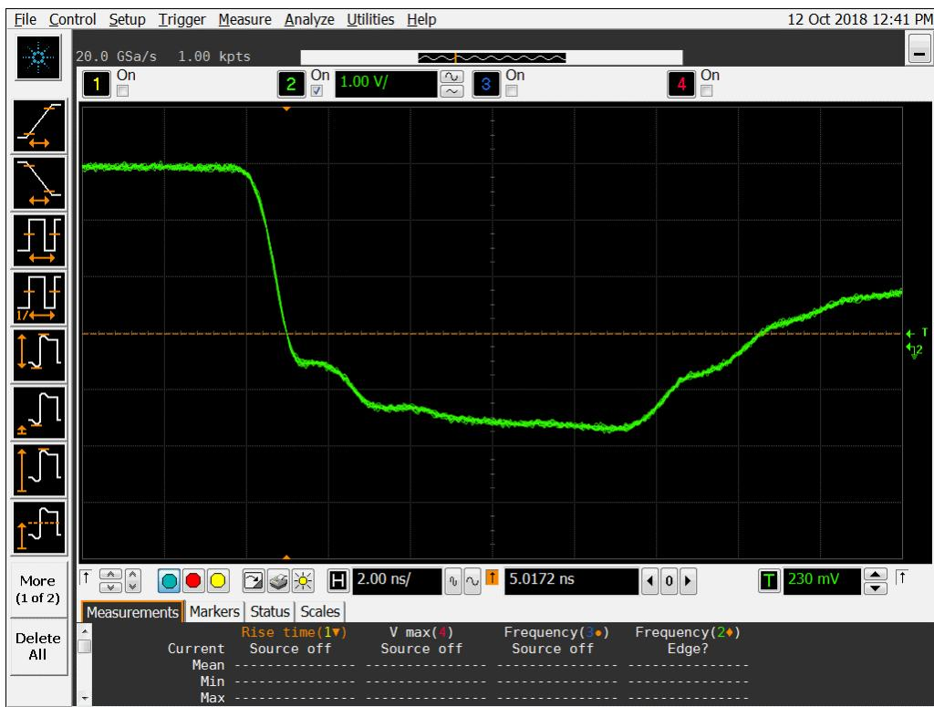
**Figure 15b DUT 7146 Post-Annealing Falling Edge.**
