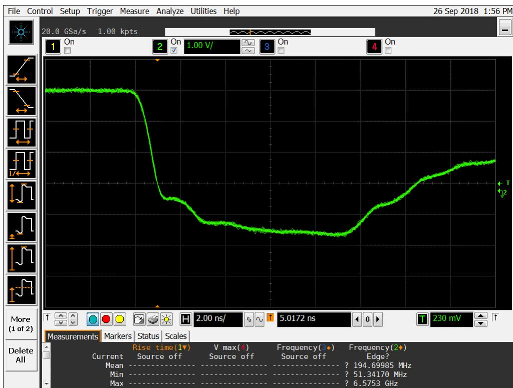
**Figure 15a DUT 7146 Pre-Irradiation Falling Edge.**
