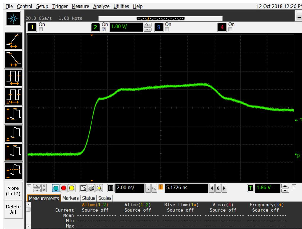
Figure 12b DUT 7111 Post-Annealing Rising Edge.
