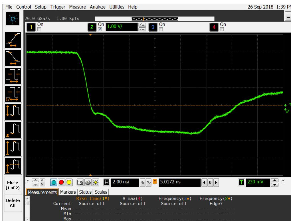
**Figure 18a DUT 7111 Pre-Irradiation Falling Edge.**
