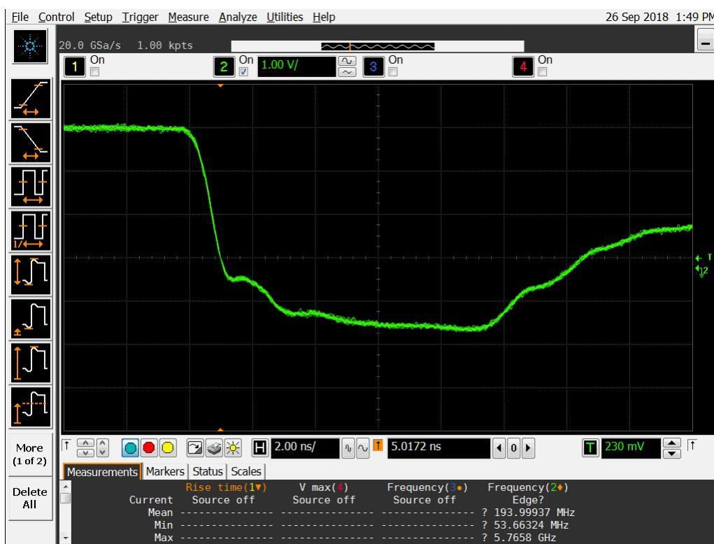
**Figure 17a DUT 7140 Pre-Irradiation Falling Edge.**
