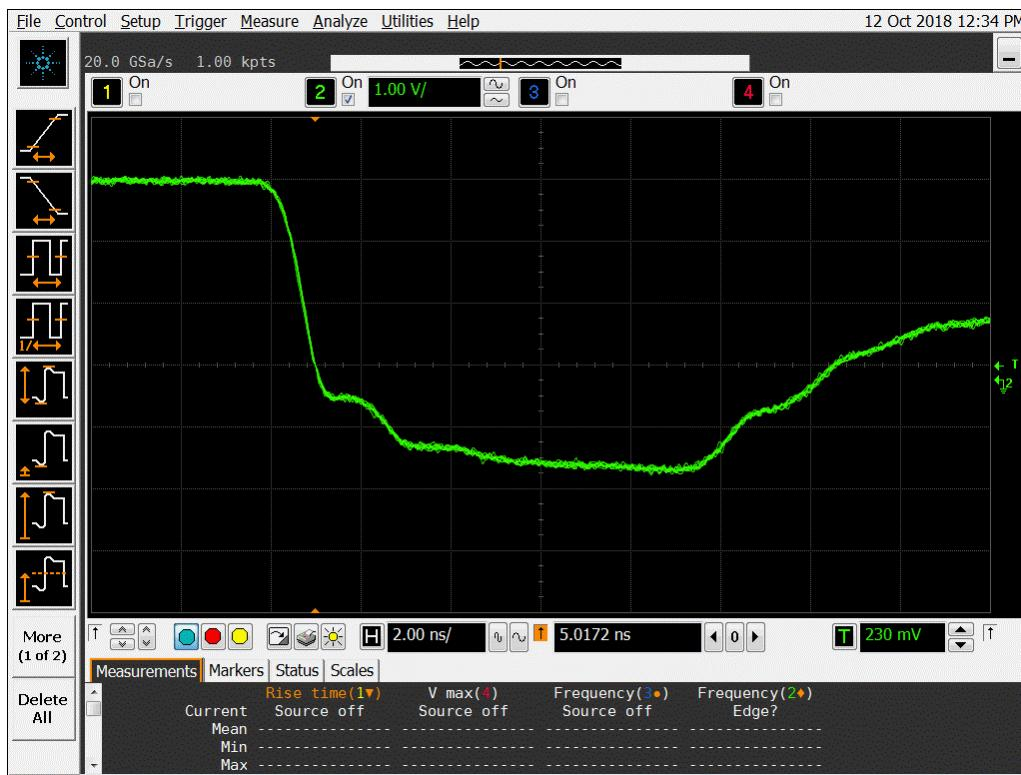
**Figure 17b DUT 7140 Post-Annealing Falling Edge.**
