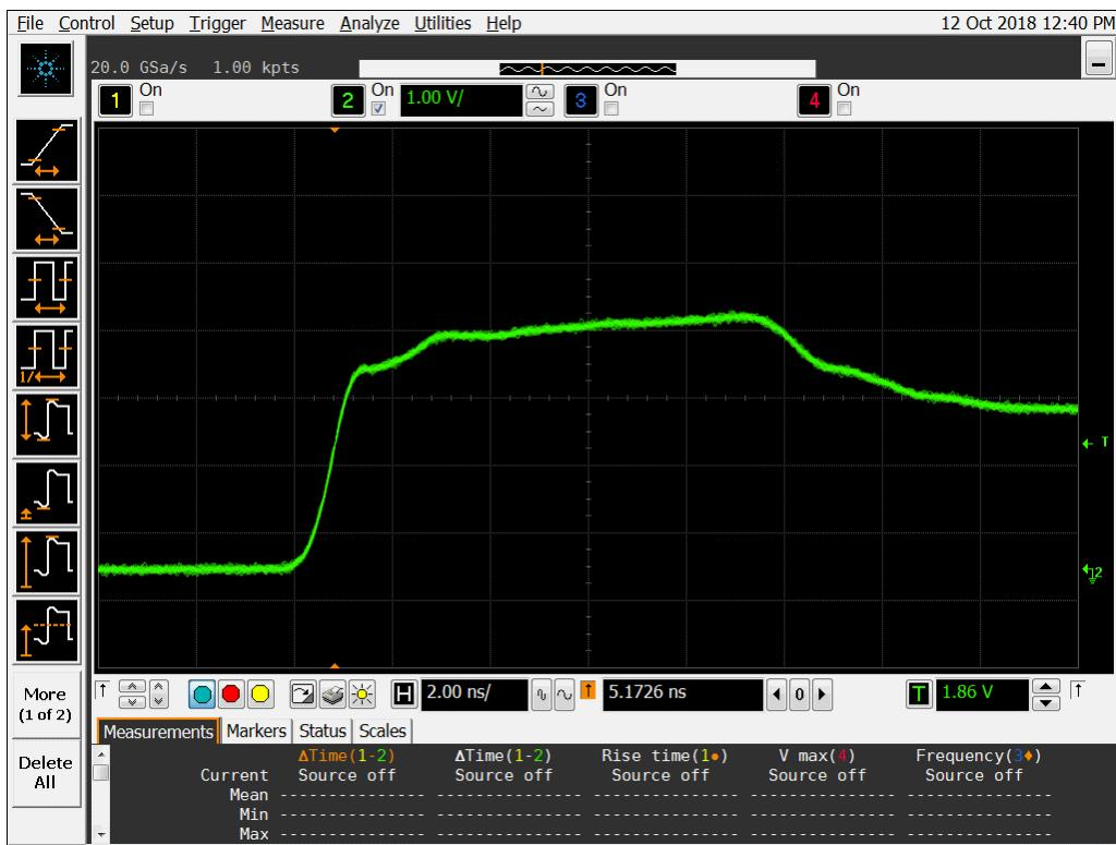
Figure 9b DUT 7146 Post-Annealing Rising Edge.
