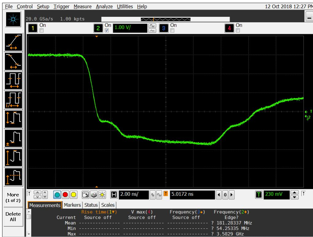
**Figure 19b DUT 7118 Post-Annealing Falling Edge.**
