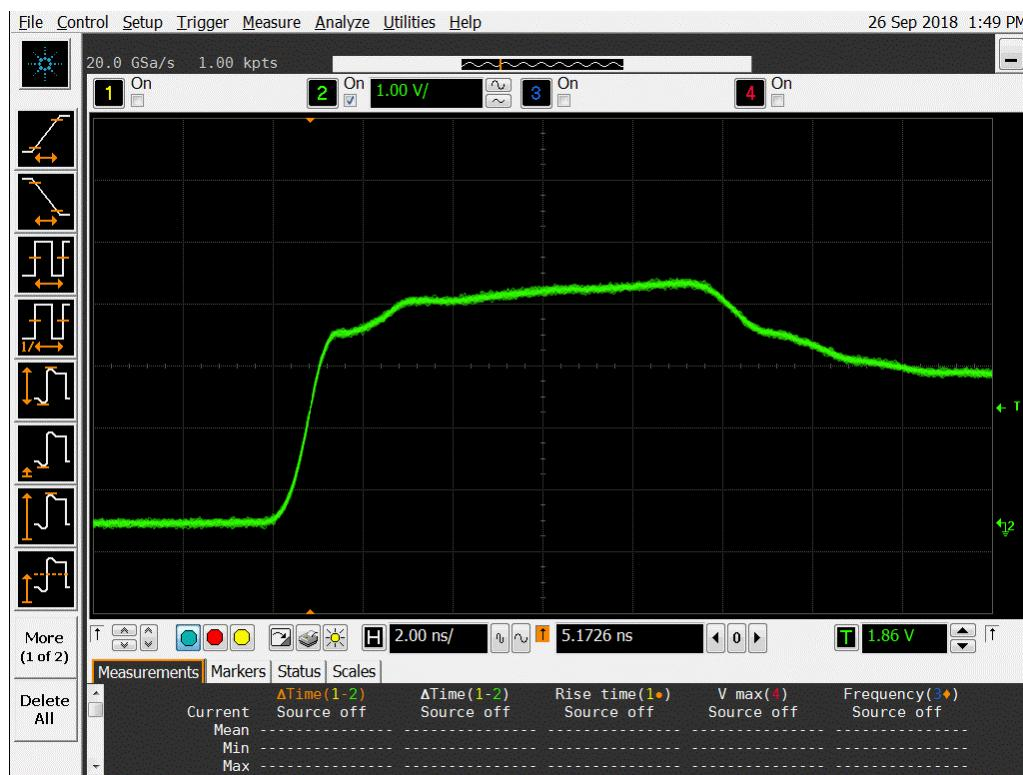
**Figure 11a DUT 7140 Pre-Irradiation Rising Edge.**
