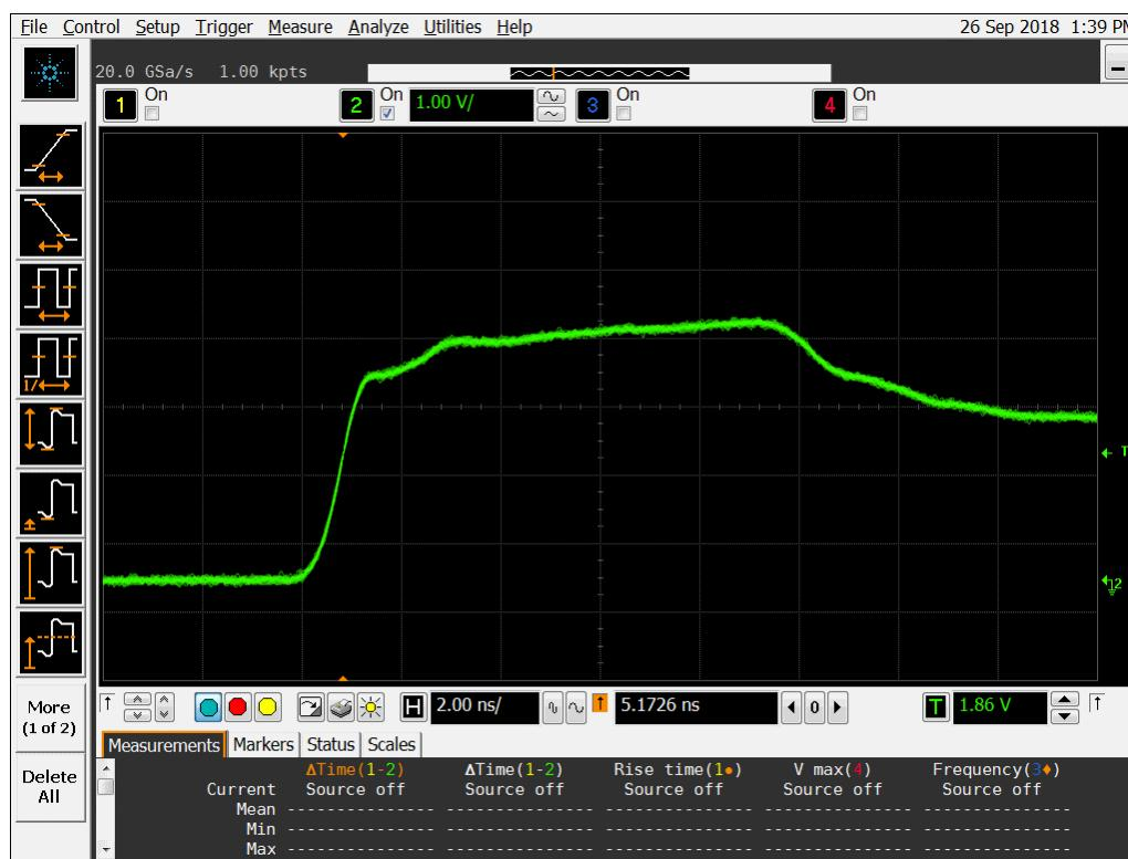
Figure 12a DUT 7111 Pre-Irradiation Rising Edge.
