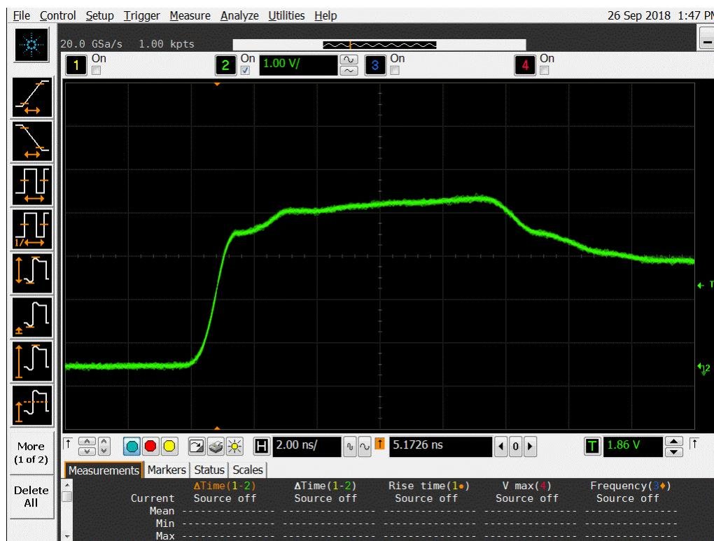
**Figure 10a DUT 7128 Pre-Irradiation Rising Edge.**
