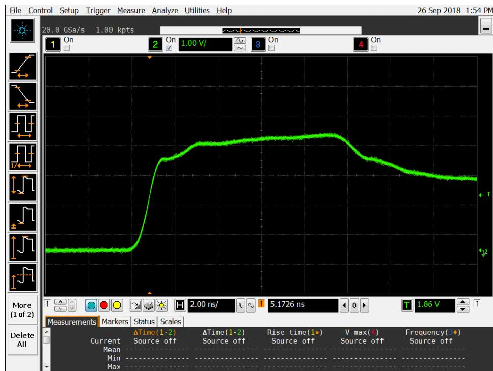
Figure 8a DUT 7141 Pre-Irradiation Rising Edge.
