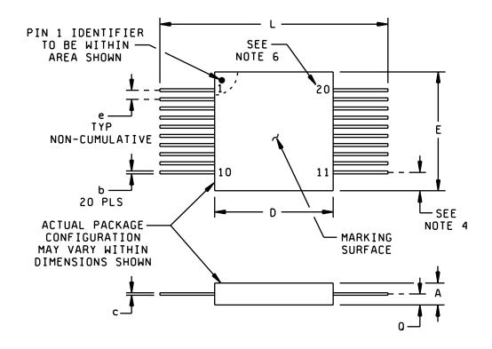
FIGURE 1. <u>Dimensions and configuration</u>.
