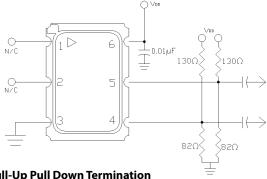
Figure 5. Pull-Up Pull Down Termination
