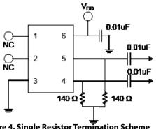
Figure 4. Single Resistor Termination Scheme
