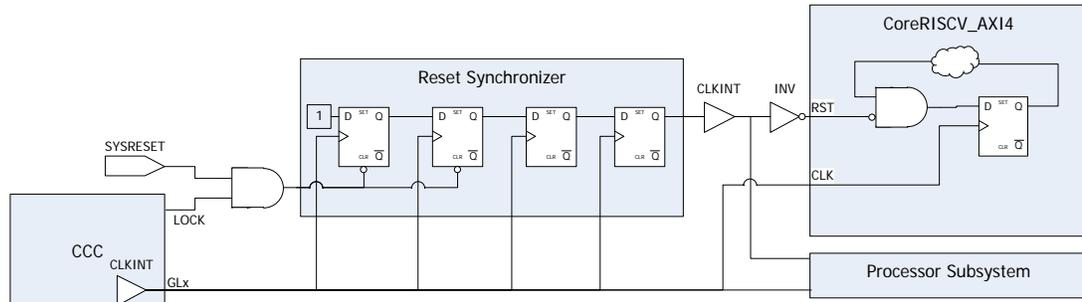
The Verilog code snippet below implements the reset synchronizer block shown in [Figure 15](#). The function of this block is to make the reset assertion and deassertion synchronous to CLK whilst guaranteeing that the reset will be seen asserted for one or more CLK cycles within CoreRISCV\_AXI4 to ensure that it is registered by all sequential elements.
