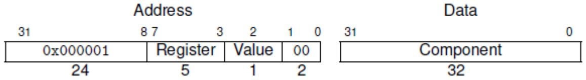
This addressing scheme was adopted so that RISC-V debug ROM routines can signal that a hart has stopped using a single store instruction to an absolute address (offset from register x0) and one free data register, which holds the hart ID.
