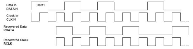
Figure 6. Clock and Data Timing Relationships for the NRZ data
