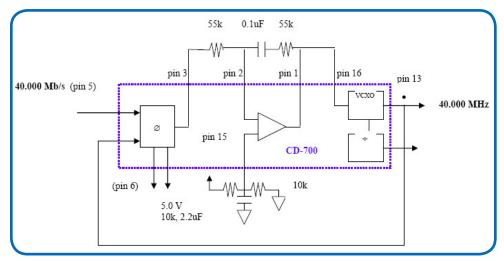
Figure 10. 40.00MHz NRZ CLock Recovery
