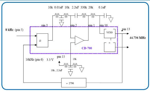
Figure 8. 8kHz to 44.736MHz Frequency Translation
