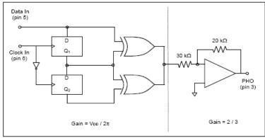
Figure 4. Simplified Phase Detector Block Diagram
