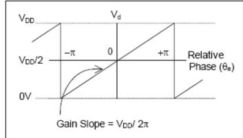
Figure 5. Open Loop Phase Detecto Transfer Curve
