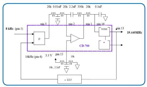
Figure 9. 8kHz to 19.44MHz Frequency Translation
