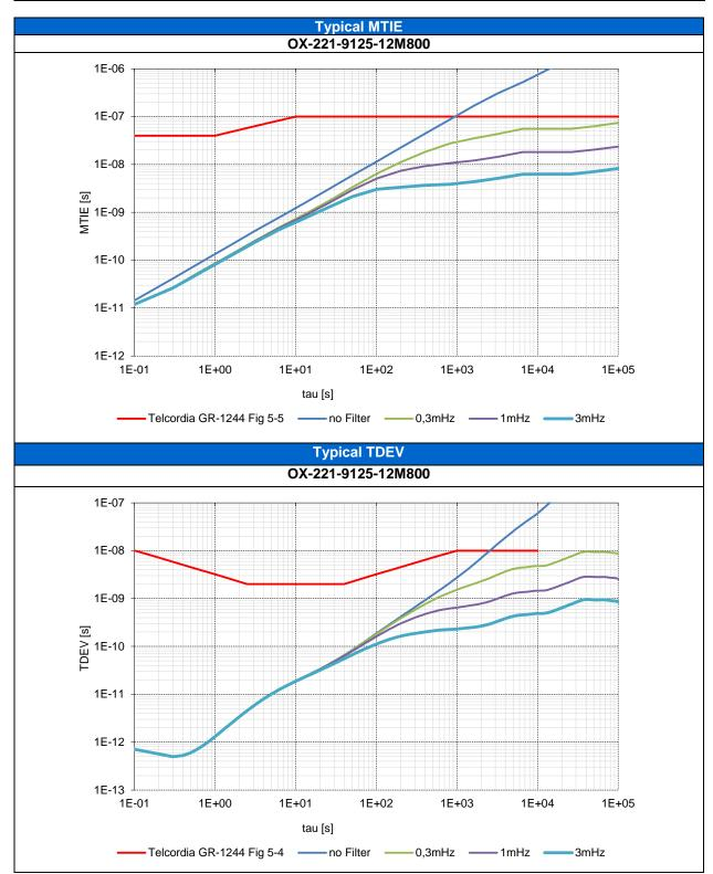
Filtered (0.3mHz, 1mHz,3mHz) curves are simulated base on measured frequency / Phase data
