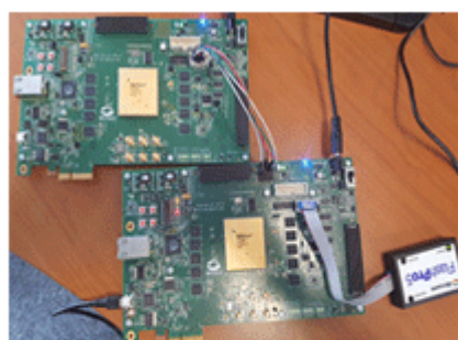
Setup of the RTG4 source board (bottom) programming the RTG4 target board (top) using DirectC v4.0 and RISC-V microprocessor
