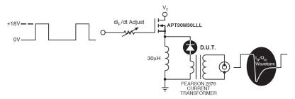
Figure 9 • Diode Test Circuit
