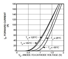
Figure 2 • Forward Current vs. Forward Voltage
