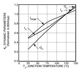
Figure 6 • Dynamic Parameters vs. Junction Temperature
