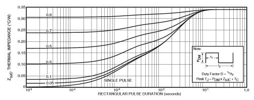
Figure 1 • Maximum Transient Thermal Impedance
