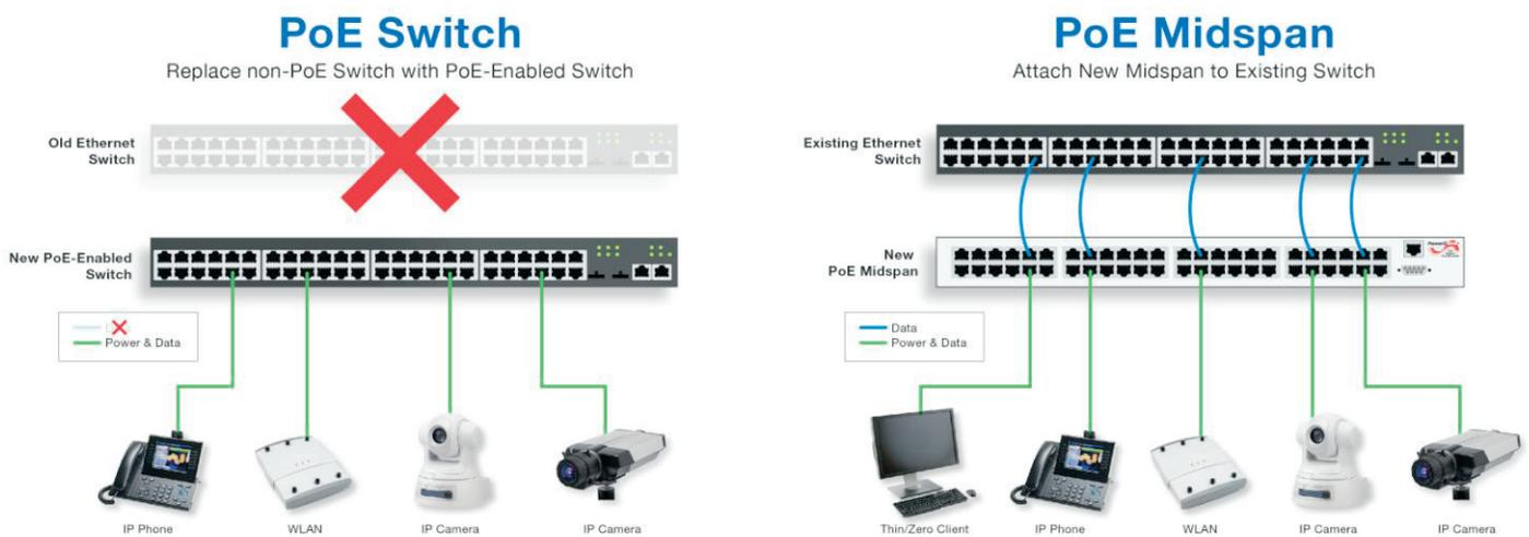
Fig. 3: Midspans offer a variety of advantages over switches for PoE deployment.
