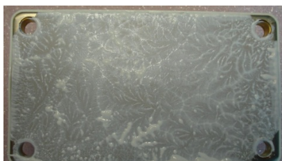
Picture 3: Grease on the module after disassembling.
