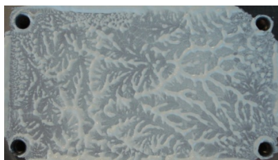
Picture 2: Grease on the heat sink after removing the module.
