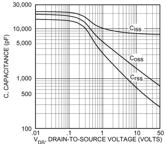
Figure 4. Typical capacitance as a function of  $v_{DS}$
