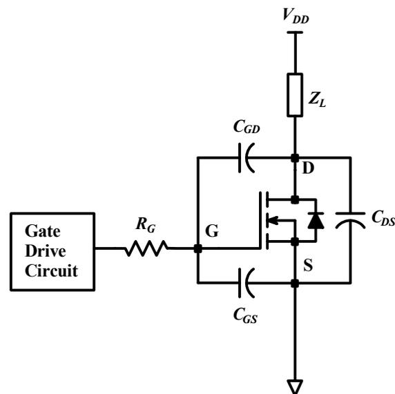
Figure 1. Lumped element model for a power MOSFET
