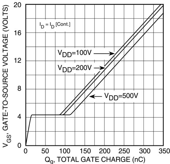
Figure 2.  $v_{GS}$  as a function of gate charge
