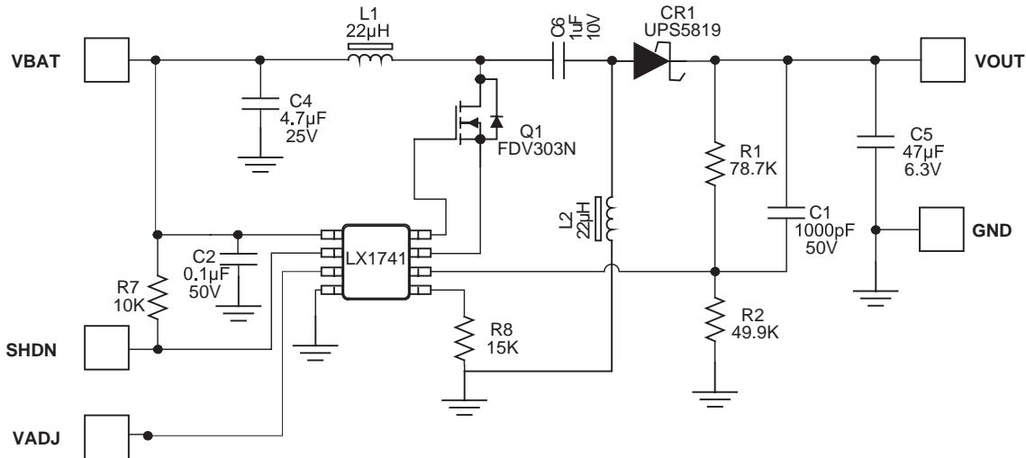
**FIGURE 13 – LX1741 SEPIC: TWO-CELL TO 3.3V
