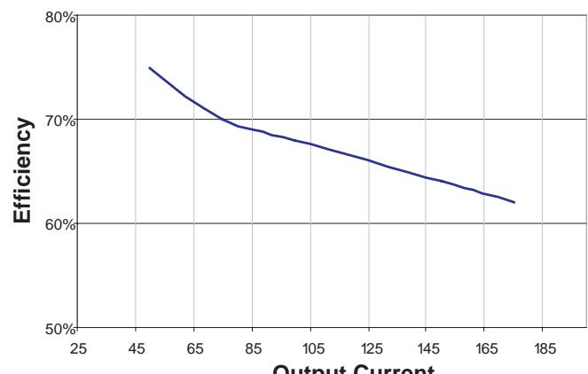
**FIGURE 18 – EFFICIENCY VS. OUTPUT CURRENT (mA)**
