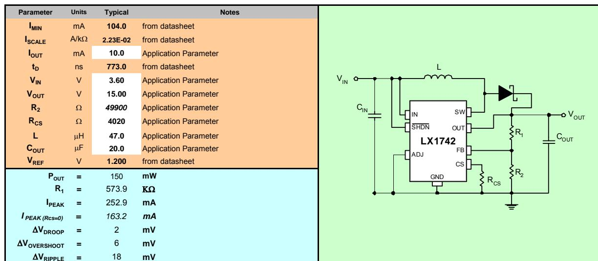
FIGURE 12 – LX1742 DESIGN CALCULATOR SPREADSHEET
