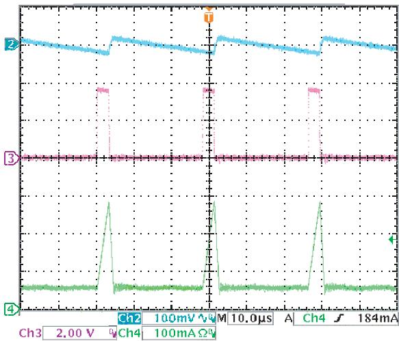
**FIGURE 10 – LX1741 WAVE FORMS  $I_{LOAD} = 5\text{mA}$**
