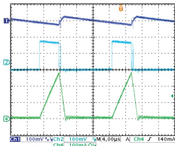
FIGURE 7B – ACTUAL SWITCHING WAVEFORMS
