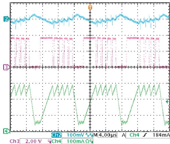
**FIGURE 11 - LX1741 WAVE FORMS  $I_{LOAD} = 40\text{mA}$**
