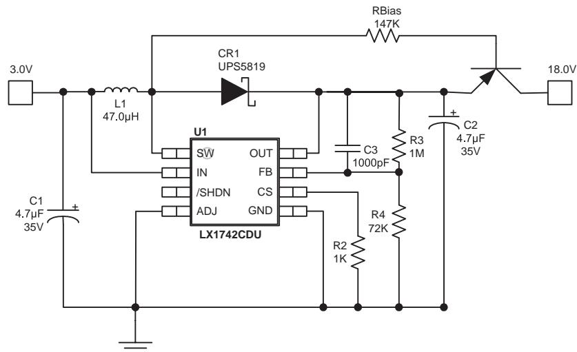
FIGURE 19 – LX7142 WITH OUTPUT DISCONNECT (2N3906)
