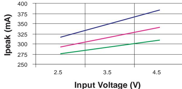
FIGURE 6 –  $I_{PEAK}$  (mA) VS. INPUT VOLTAGE
