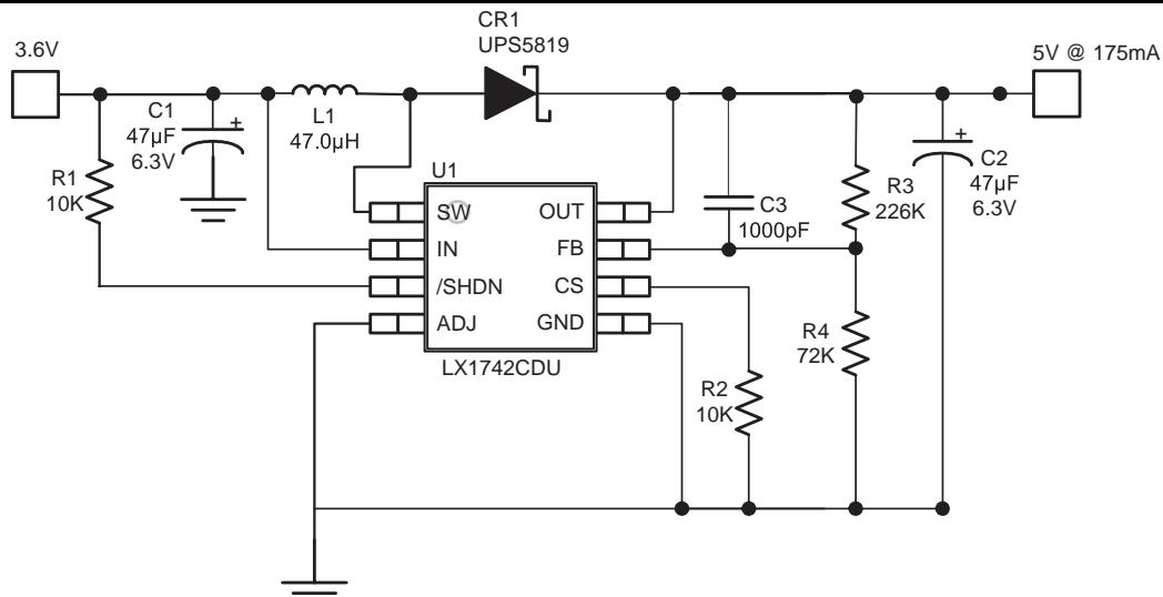
**FIGURE 16 – LX1742 3.6V TO 5V Boost (175mA)**
