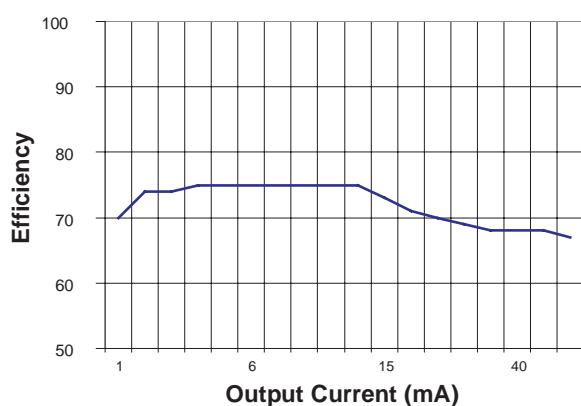
FIGURE 4 – LX1742 EFFICIENCY VS. OUTPUT CURRENT
