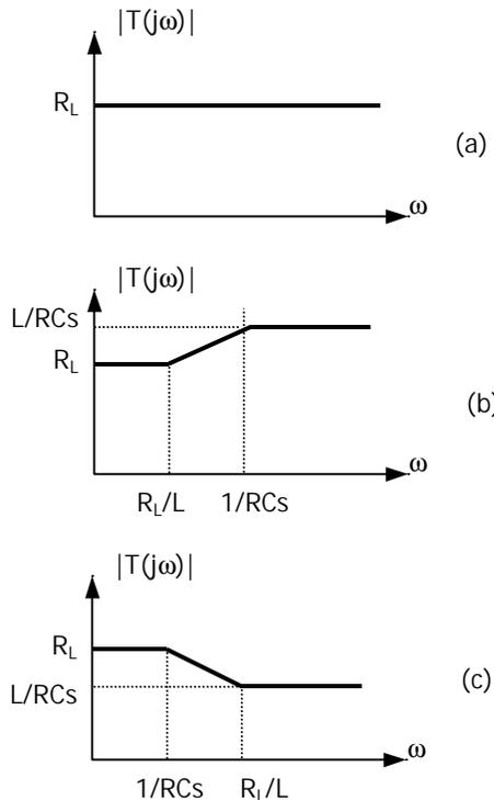
Figure 4 - The gain of the new current sensor. (a)  $L/R_L = RC_s$ ; (b)  $L/R_L > RC_s$ ; (c)  $L/R_L < RC_s$
