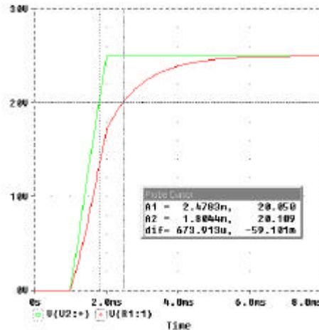
Figure 6(a) - Response to a 25A step current when  $L/R_L < RC_s$
