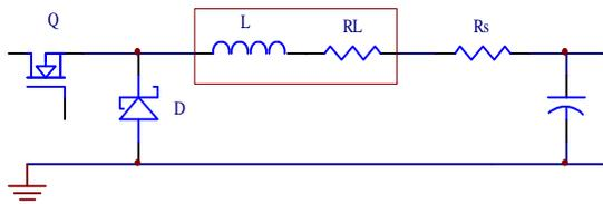
Figure 1 – A buck converter with a resistor  $R_s$  for sensing the inductor current. The resistor  $R_L$  is the parasitic resistance of the inductor.
