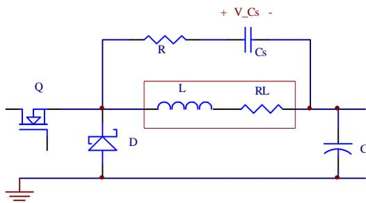
Figure 2 - The new current sense technique
