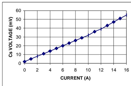
Figure 9 - The measured Cs voltage versus inductor current
