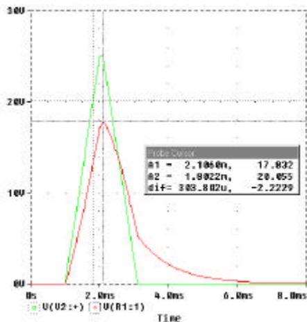
Figure 6(b) - Response to short duration transient
