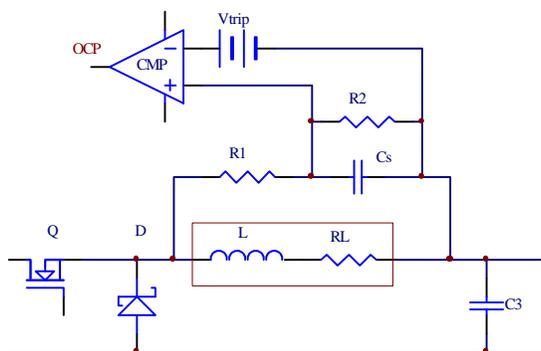
Figure 8(a) - Complete Sense Circuit
