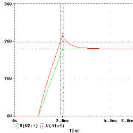
Figure 5 - The response of the current sensor to an 18A step current in the inductor when  $L/R_L > RC_s$
