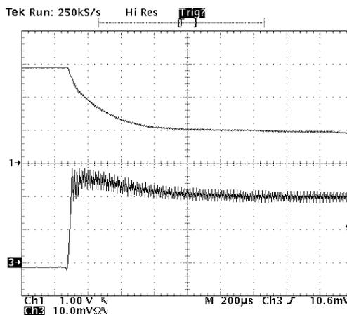
Figure 10 - OCP Action. The top trace is output voltage (1V/div) and the bottom is inductor current (10A/div)
