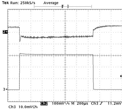
Figure 11 - Step load response. Top trace is output voltage (100mV/div) and bottom is load current (5A/div)
