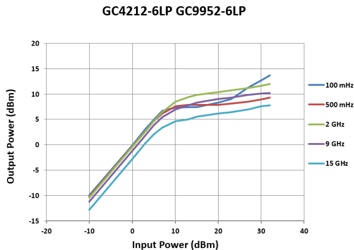
Figure 8 • GC4212-6LP and GC9952-6LP CW Multi-Stage Transfer Characteristics
