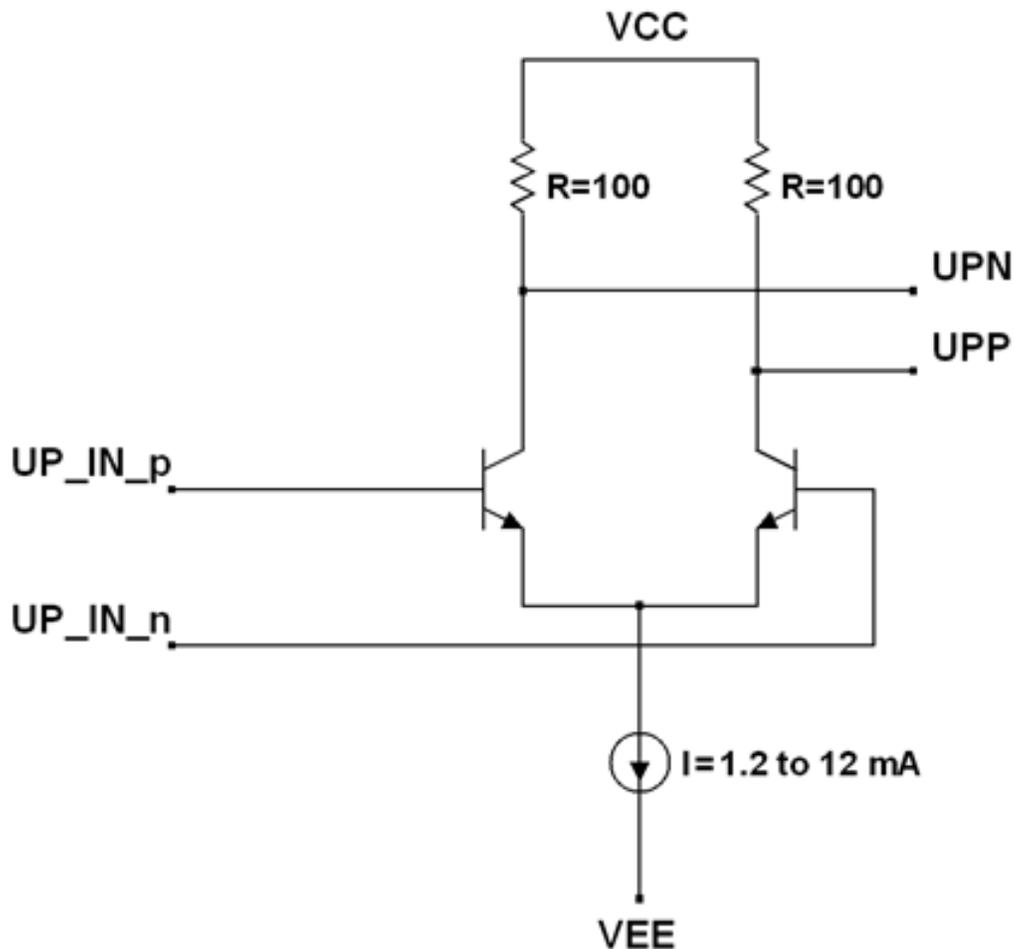
*Simplified Charge Pump Output Circuit*
