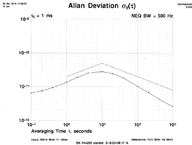
Figure 9: 100 MHz LNCSAC Allan Deviation
