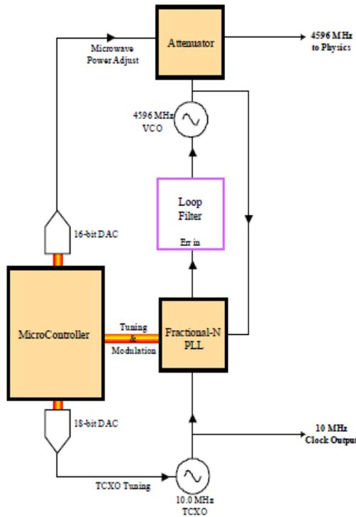
Figure 3: CSAC Microwave Subsystem
