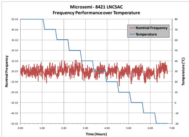
Figure 6: LNCsAC Frequency vs Temperature
