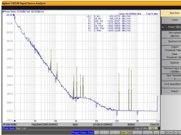
Figure 8: 100 MHz LNCSAC Phase Noise
