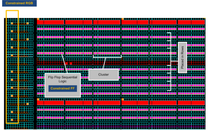
Fig. 3 Designer layout shows the place and route of FFs in a shift register to assure them controlled by the same RGB.
