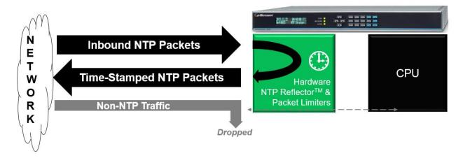
The NTP Reflector® protects the time server from excessive network traffic and denial of service (DoS) attacks, while simultaneously providing extremely high-bandwidth, high-accuracy NTP server operations. The Reflector is a real-time, hardware-based NTP packet identification and time stamping engine. Received NTP client packets are identified at line speed, precise and accurate T2 and T3 time stamps are added and the packet is returned to the requesting NTP client.
