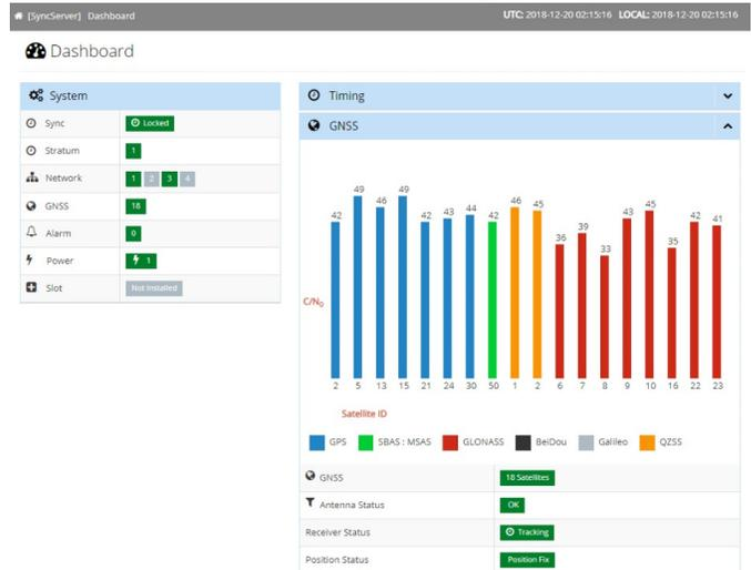
*Tracking multiple constellations significantly improves the overall number of visible satellites available to continuously derive the time.*
