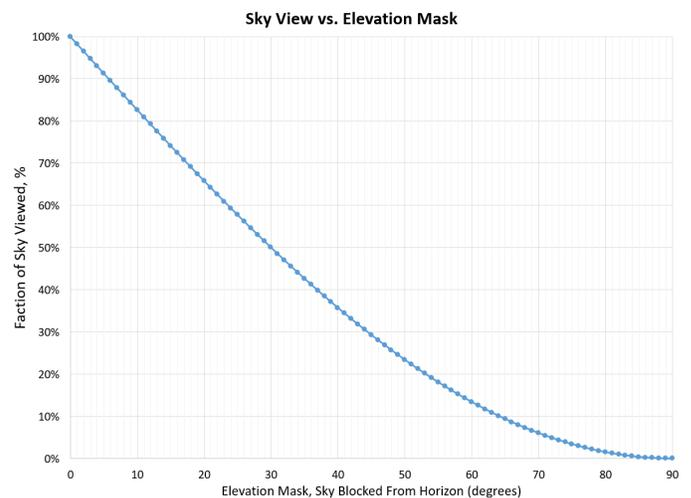
*An elevation mask, much like urban canyon environments, eliminates multipath-prone low-elevation satellites, but also limits the amount of sky that can be seen to track remaining satellites.*
