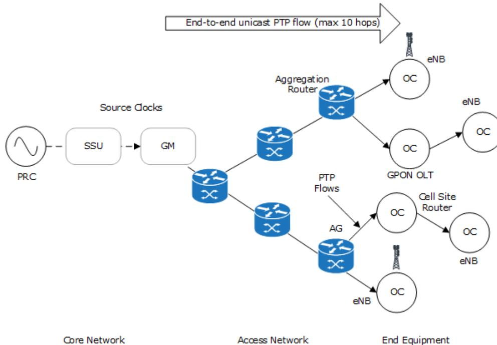
**Note:** A grandmaster (GM) clock is a PTP server and an ordinary clock (OC) is a PTP slave/client.
