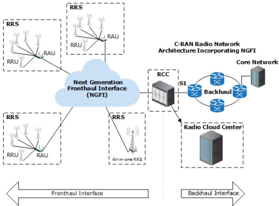
The current mobile backhaul architectures in place today have alternative solutions for meeting the timing requirements (frequency, time, and phase) documented in the industry standards. These requirements are evolving to support the evolution from LTE to LTE-TDD and LTE-Advanced technologies.
