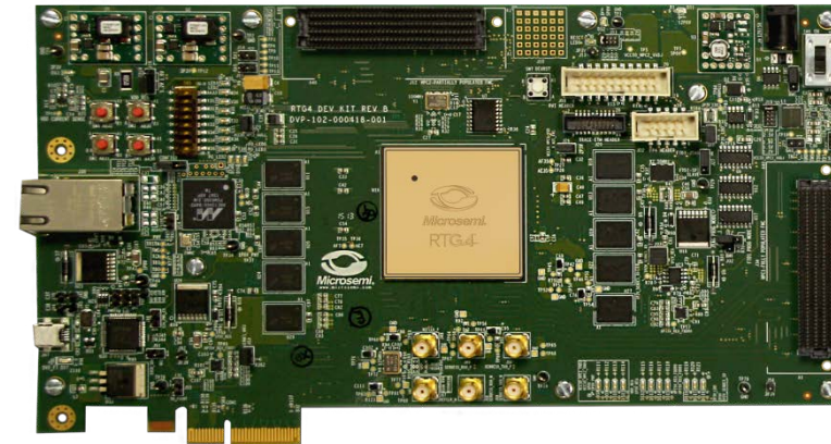
RTG4 Dev Kit #2 hosts RTG4 to be reprogrammed by RTG4 Dev Kit #1
