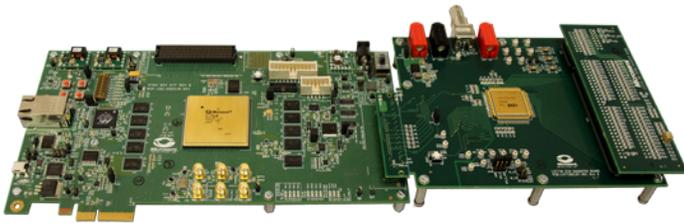
high-performance FPGAs. The development board features a RT4G150 device offering more than 150,000 logic elements in a ceramic package with 1,657 pins.
