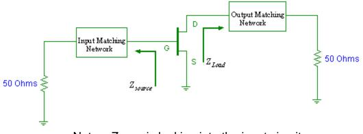
Note:  $Z_{Source}$  is looking into the input circuit  $Z_{Load}$  is looking into the output circuit
