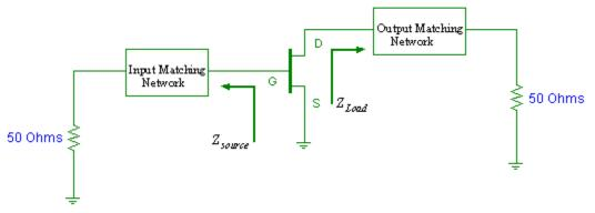
Note:  $Z_{Source}$  is looking into the input circuit;  $Z_{Load}$  is looking into the output circuit.
