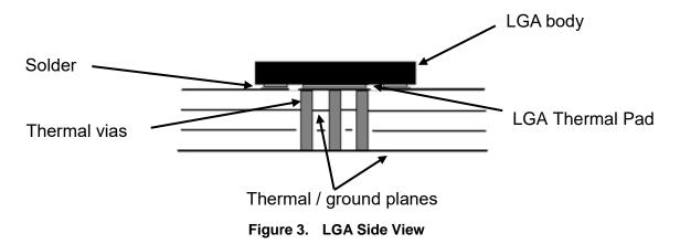
The recommended package land layout is provided in the individual product datasheets. Use of small or filled vias under the thermal paddle prevents wicking of solder from under the part; open vias larger than .010" - .012" in diameter will wick solder away from the PC board thermal pad and should be avoided.
