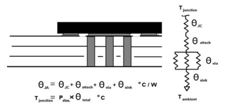
Figure 5. PC board heatsink thermal model
