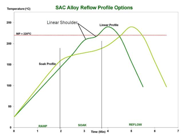
Figure 4. Typical solder reflow profile for SAC305 type of solder paste (courtesy of Indium Corp.)
