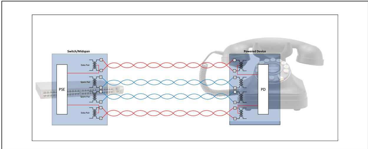
The next illustration (Figure 2) shows a four-pair power connection where power is delivered over all 8 wires.
