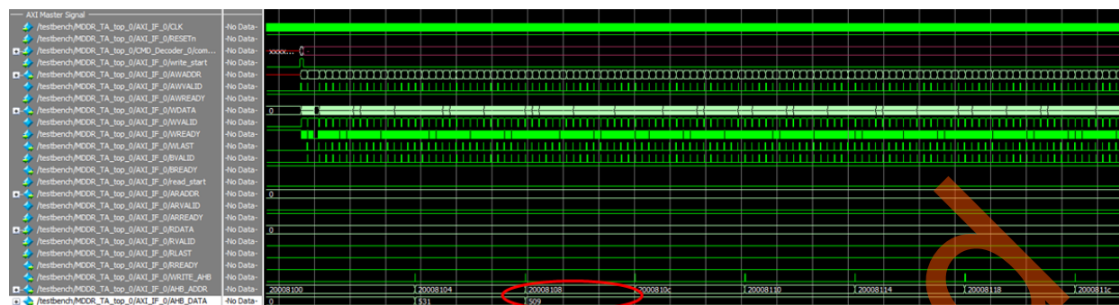
Figure 17 • AXI Master (AXI_IF) Signals for Write Operation
