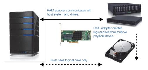
Each logical drive that the RAID adapter creates has data protection built into it in the form of a RAID level. The level of RAID assigned to an individual logical drive depends on the number of physical drives included (some RAID levels require minimum and/or maximum numbers of drives) and whether system performance or data security is the priority.
