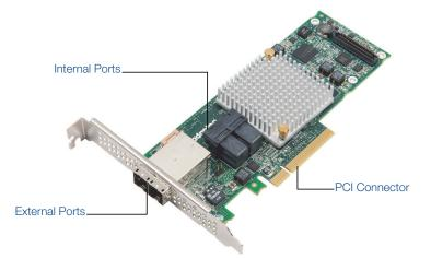
A RAID adapter sits in the center of the input/output (I/O) path, communicating data from the host system to the storage devices and vice versa, taking on the tasks of storing and retrieving data that are otherwise done by the host system's microprocessor (CPU). It does not rely on the host system for resources, instead freeing up the CPU to run applications.
