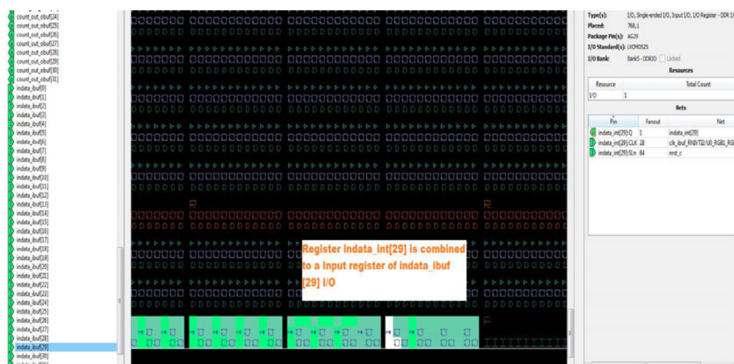
Figure B-1 • Register Combined with Input Register of an I/O
