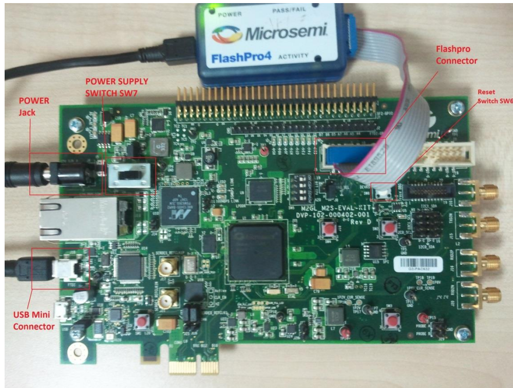
Figure 4. SmartFusion2 Security Evaluation Kit Board Setup
