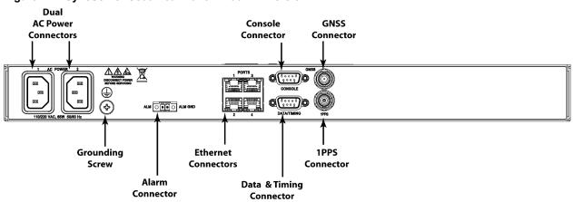
Figure 1-4. SyncServer S600 Rear Panel - Dual AC Version
