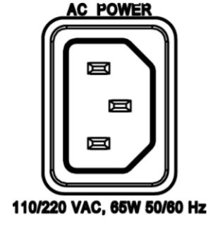
Figure 2-7. SyncServer S6x0 Single AC Power Connector
