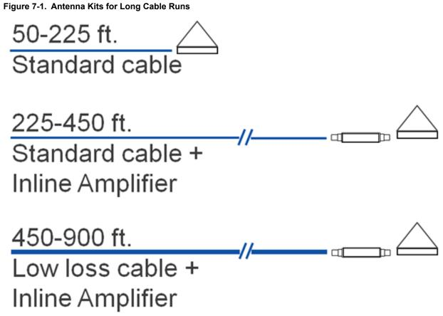
The antenna kit (part number 093-15202-001) includes a short SyncServer adapter cable (part number 060-00039-000) with BNC(m)-N(f) connectors. All primary antenna cables use N(m) connectors on either end. A single cable must be used between the adapter cable and the next accessory (lightning arrestor, inline amplifier, or antenna). Lightning arrestors include a 25 ft. cable to connect to the next accessory (inline amplifier or antenna).
