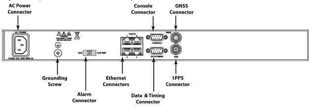
Figure 1-3. SyncServer S600 Rear Panel - Single AC Version with 10 GbE
