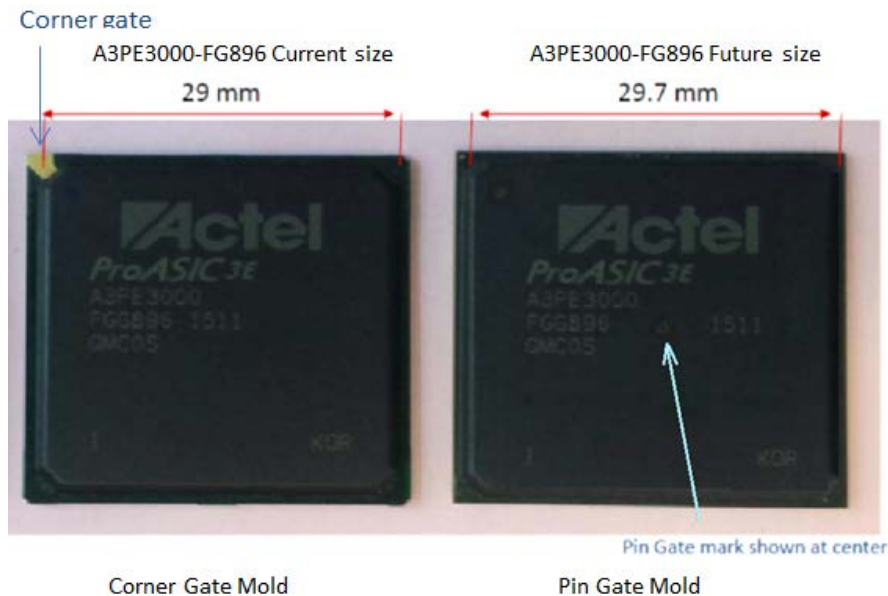
Figure 1 Comparison of FGG896 Packages with CGM (Left) and PGM (Right) Mold
