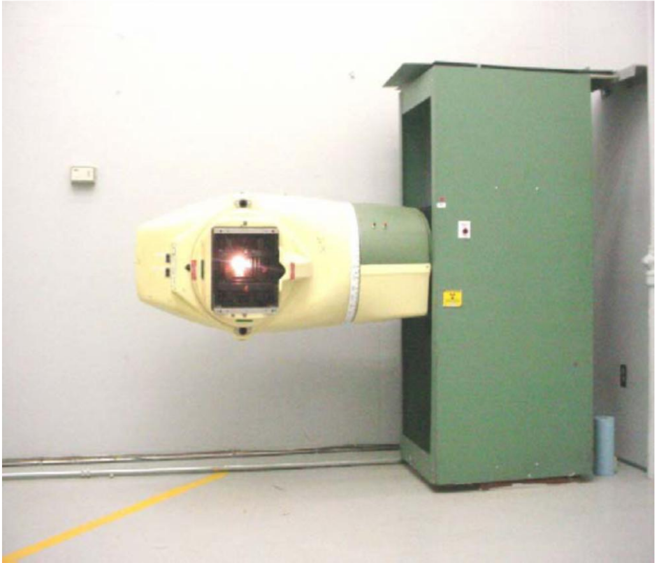
Figure 2.1. The "Eldorado" low-dose irradiator at the El Dorado Irradiator Facility of the SVAD White Sands Missile Range in New Mexico provided the Co60 gamma rays for this testing.
