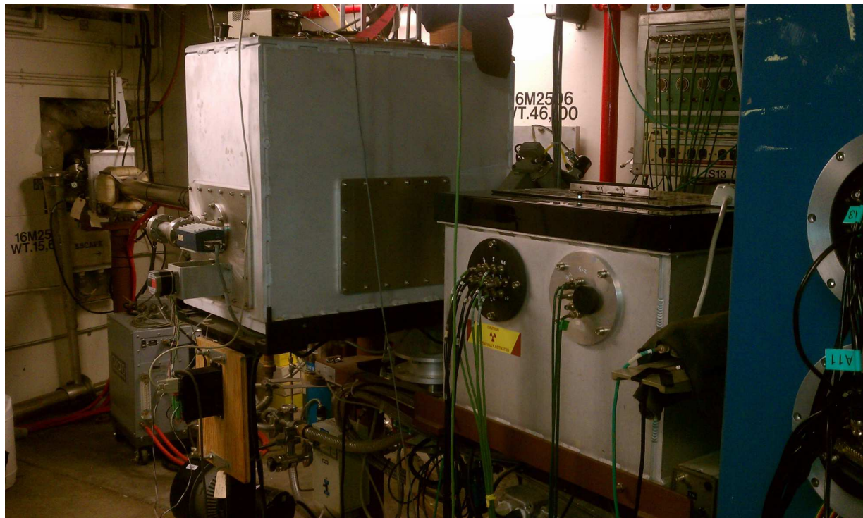
Figure 5. Photograph of beam line attached to chamber with feed-throughs on right.
