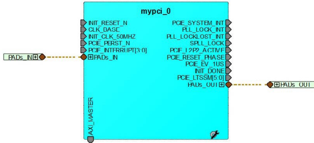
Figure 1-4. mypci Block Instantiation on the SmartDesign Canvas
