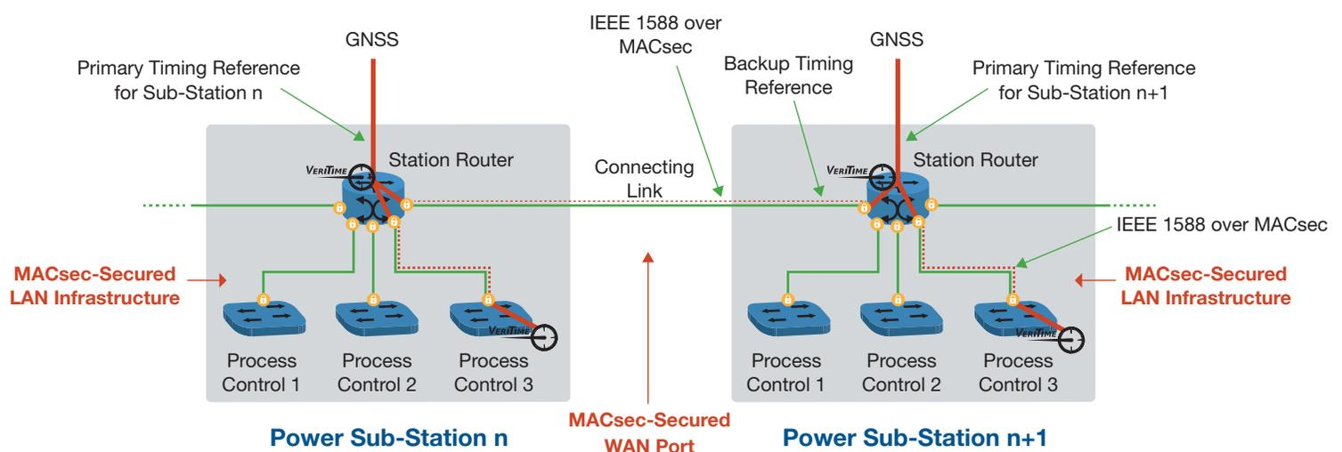
Figure 1. Using PTP over MACsec in a power sub-station application
