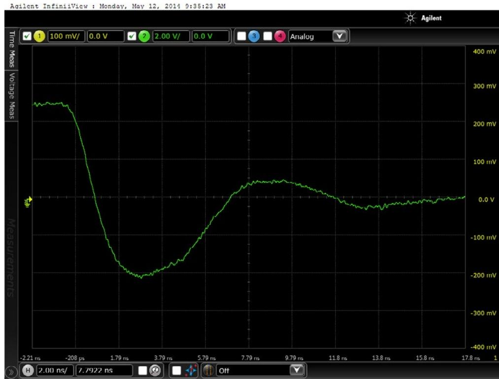
**Figure 15a DUT 3685 Pre-Radiation Falling Edge**
