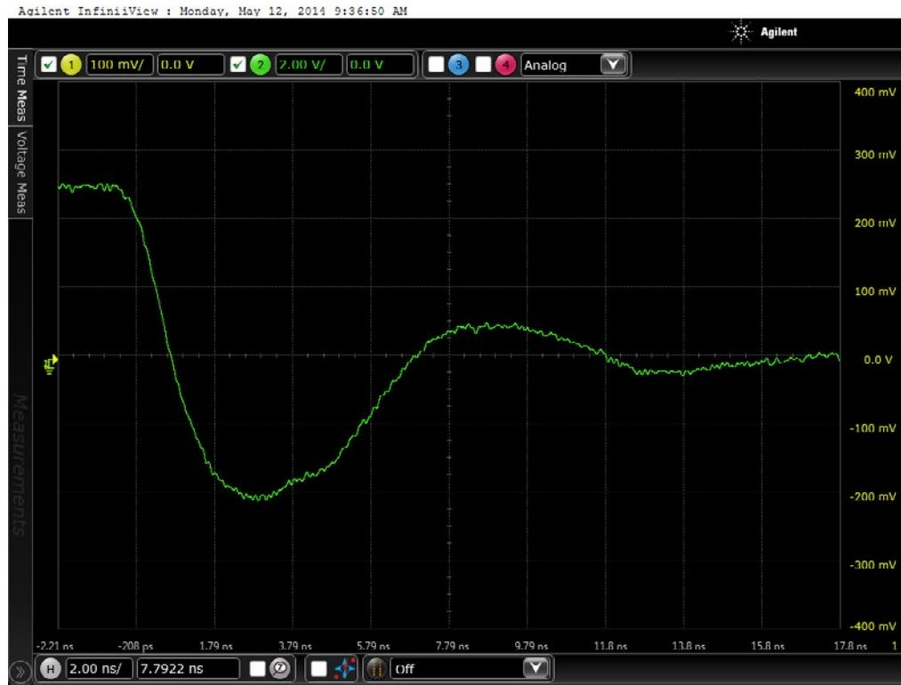
Figure 19a DUT 3822 Pre-Irradiation Falling Edge
