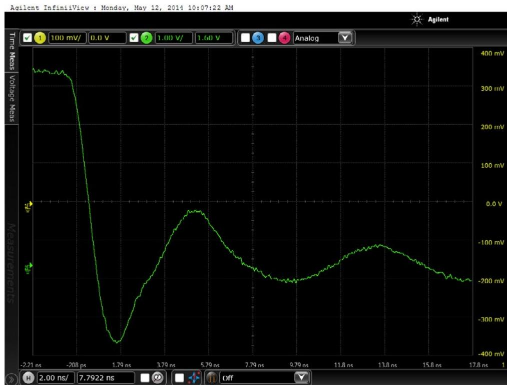
**Figure 15b DUT 3685 Post-Annealing Falling Edge**
