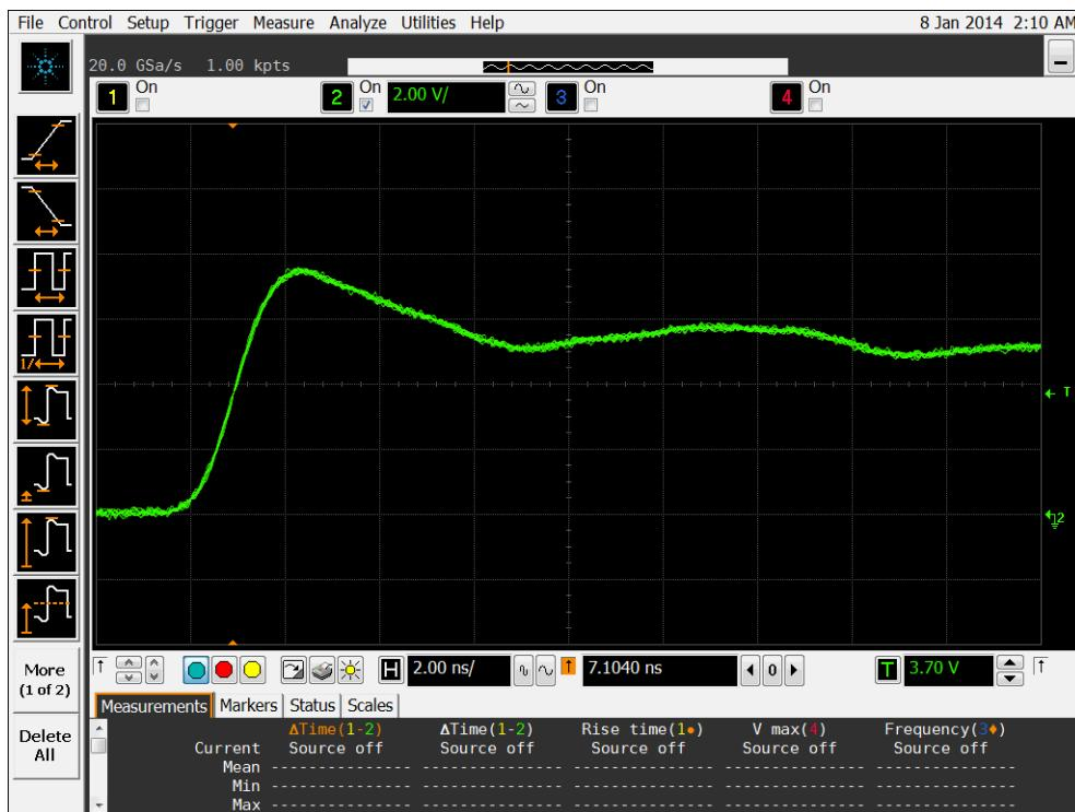
Figure 7b DUT 5388 Post-Annealing Rising Edge
