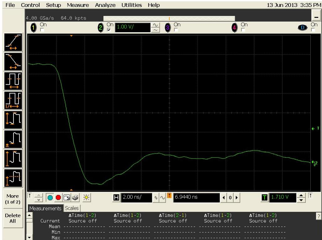
Figure 13a DUT 5501 Pre-Irradiation Falling Edge
