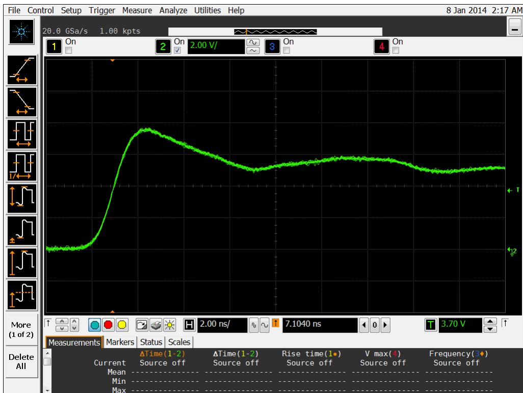
Figure 9b DUT 5504 Post-Annealing Rising Edge
