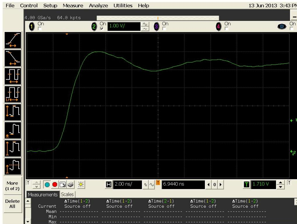
Figure 10a DUT 5608 Pre-Irradiation Rising Edge
