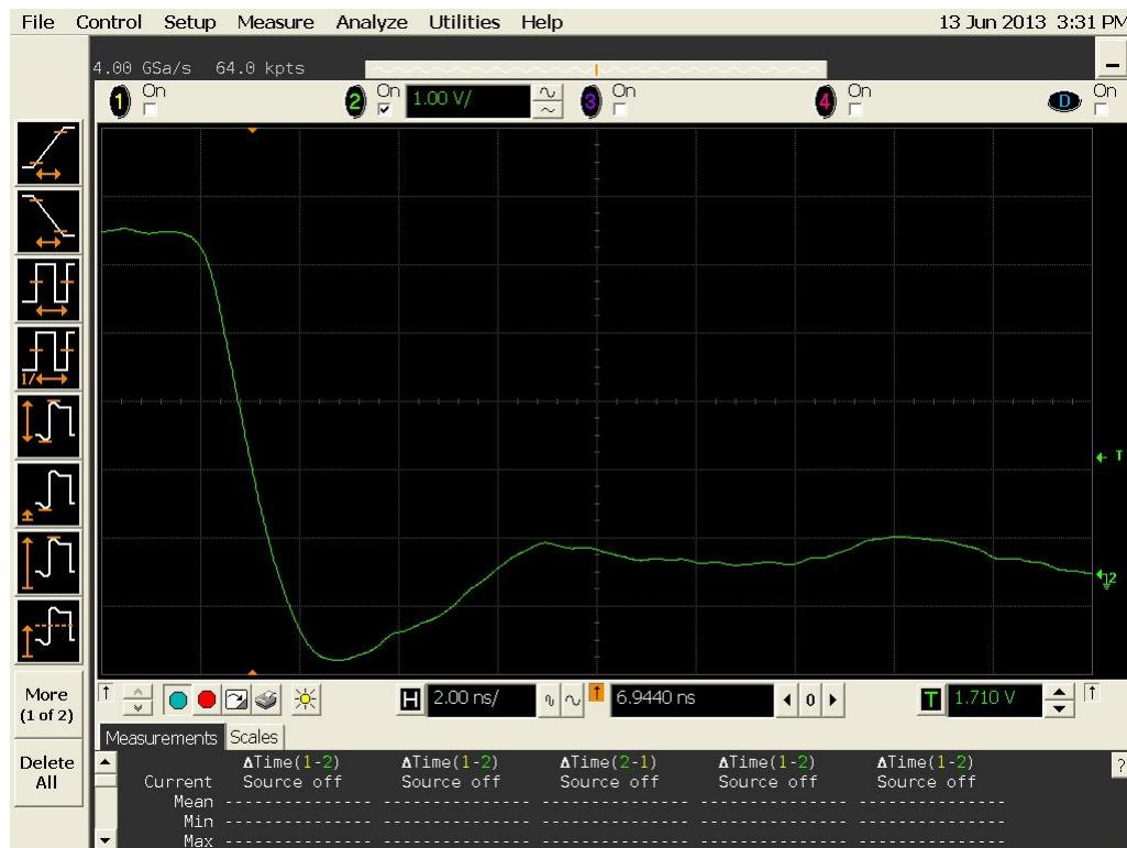
Figure 12a DUT 5388 Pre-Radiation Falling Edge
