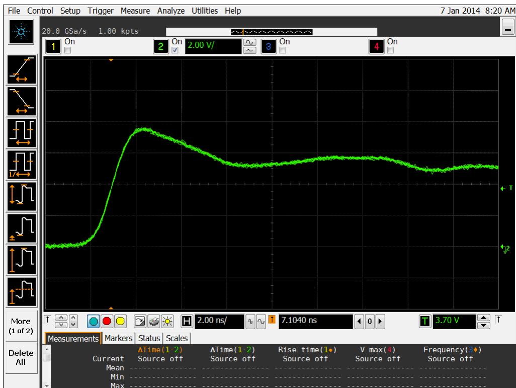
Figure 11b DUT 5629 Post-Annealing Rising Edge
