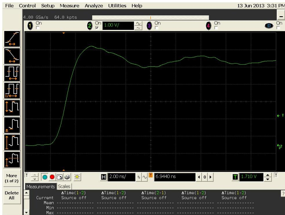
Figure 7a DUT 5388 Pre-Irradiation Rising Edge
