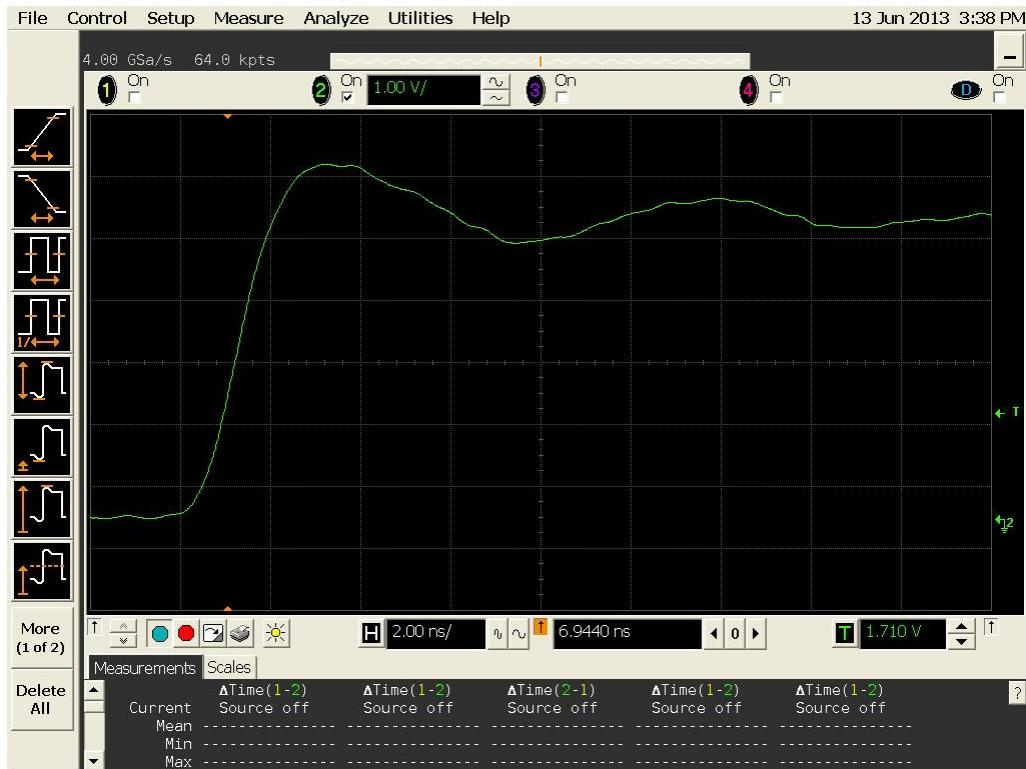
Figure 9a DUT 5504 Pre-Radiation Rising Edge
