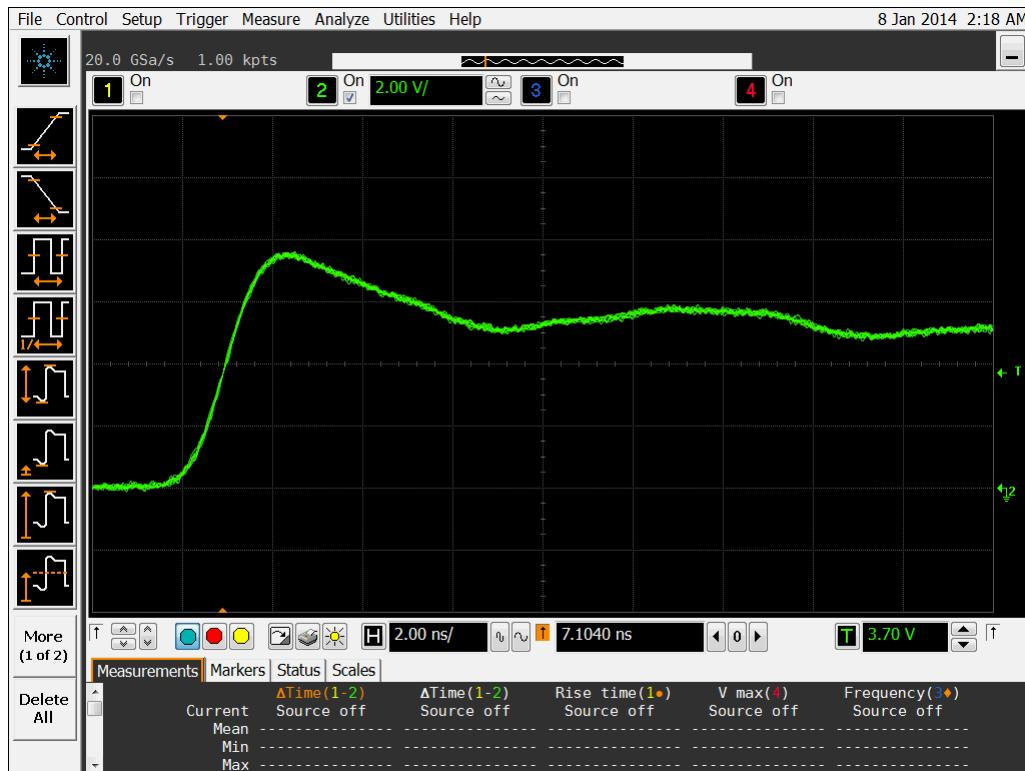
Figure 8b DUT 5501 Post-Annealing Rising Edge
