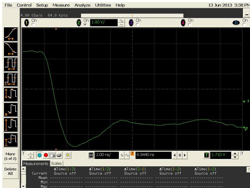
Figure 14a DUT 5504 Pre-Irradiation Falling Edge
