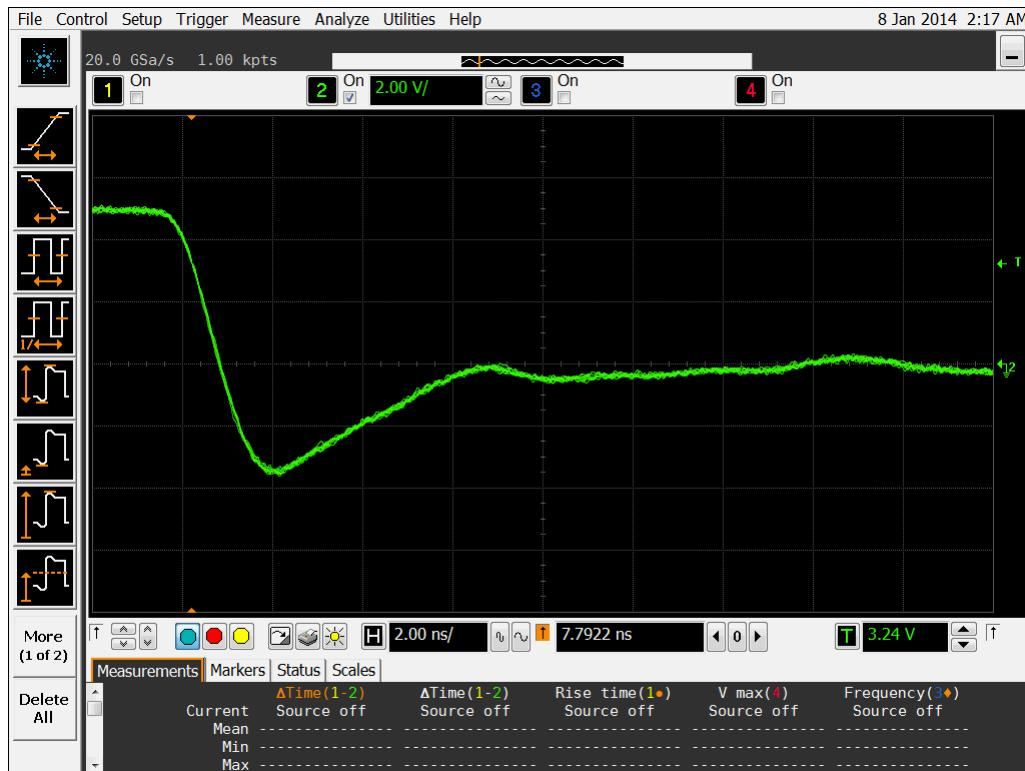
Figure 14b DUT 5504 Post-Annealing Falling Edge
