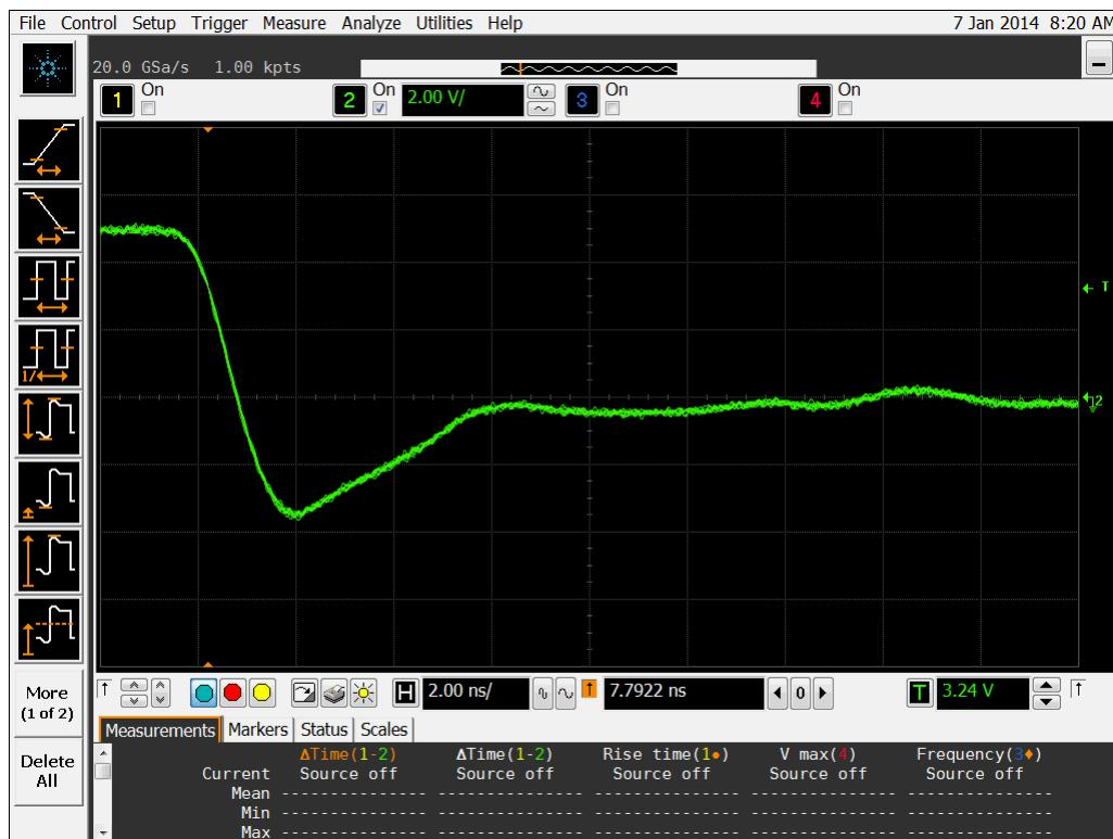
Figure 16b DUT 5629 Post-Annealing Falling Edge
