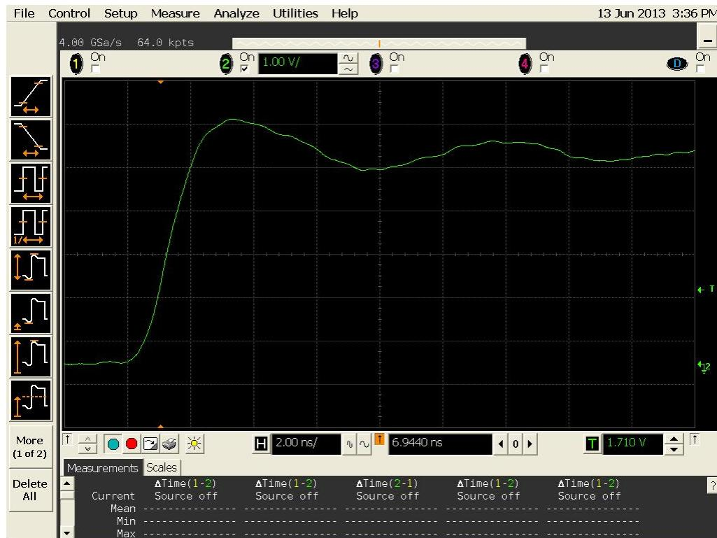
Figure 8a DUT 5501 Pre-Irradiation Rising Edge
