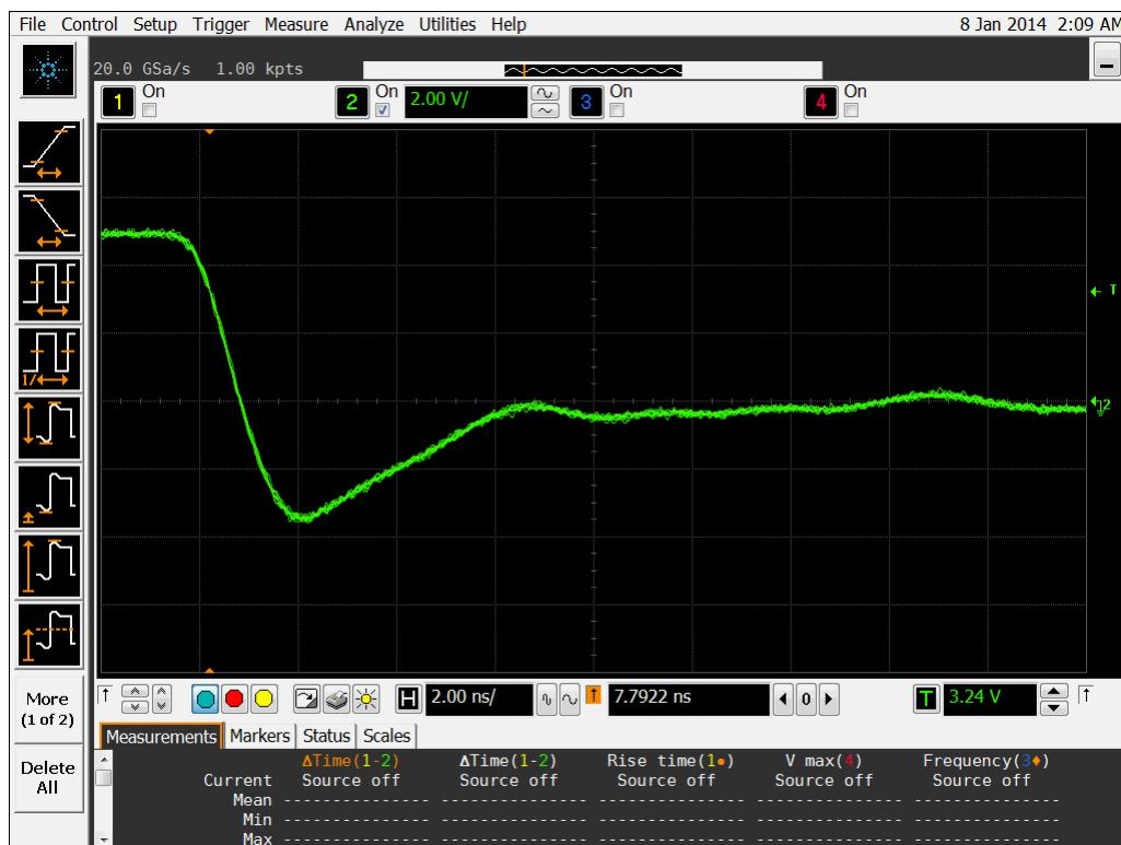
Figure 12b DUT 5388 Post-Annealing Falling Edge
