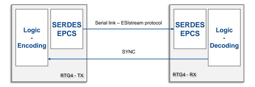
The ESIstream protocol can be used with Microsemi FPGAs to increase the efficiency of a serial interface.
