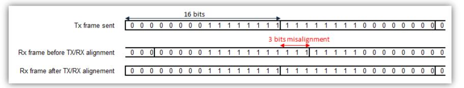
To correct frame misalignment, TX sends a known sequence for 32 frames used by RX to align its 16bits word to the TX frames.
