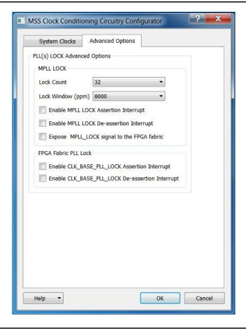
Figure 2-1 • Advanced Options Configuration Tab
