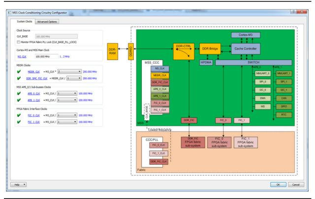
Figure 1 • MSS CCC Configurator
