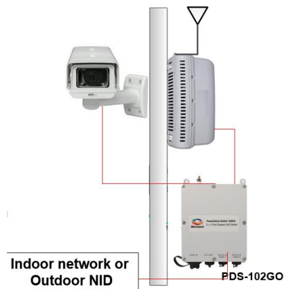
Figure 5 Wi-Fi mesh hotspot with IP camera deployment with managed PoE switch
