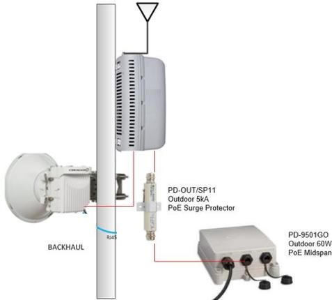
**Figure 2** deploying a power forwarding Small Cell + Backhaul with an outdoor Midspan
