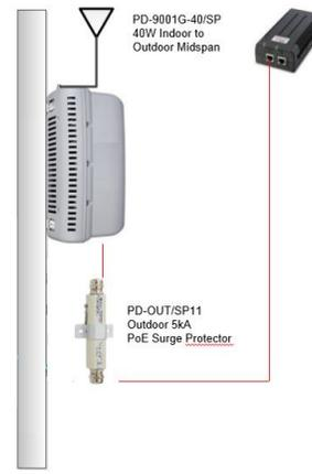
**Figure 3** Indoor to Outdoor Small Cell/Wi-Fi Hotspot Deployment
