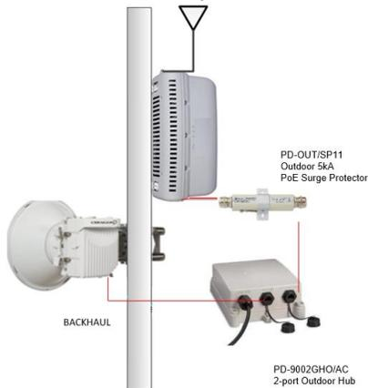
**Figure 4** Small Cell + Backhaul Deployment with PoE Hub
