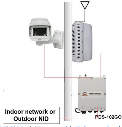
**Figure 5** Wi-Fi Mesh Hotspot with IP Camera Deployment with Managed PoE Switch
