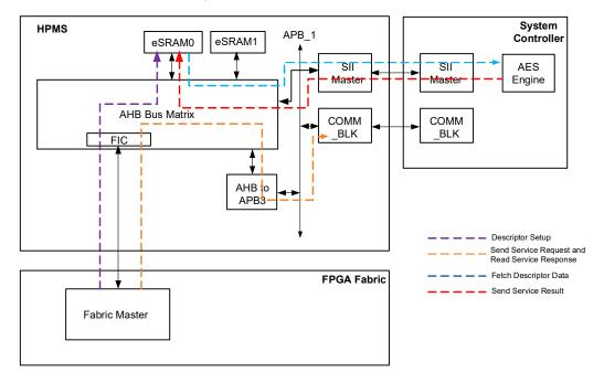
Microsemi provides a system service driver and CoreSysServices soft IP to run the SHA-256 operation in SmartFusion2 and IGLOO2. So, it is not required to write software code from scratch or create a complex master in fabric to run the SHA-256 system services.
