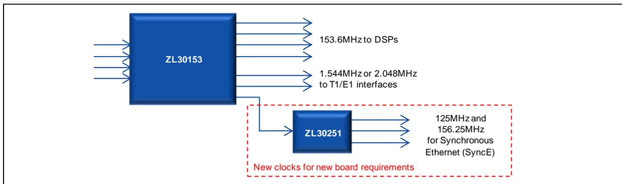
Figure 3 - Add-On Frequency Conversion Using Microsemi's ZL30251
