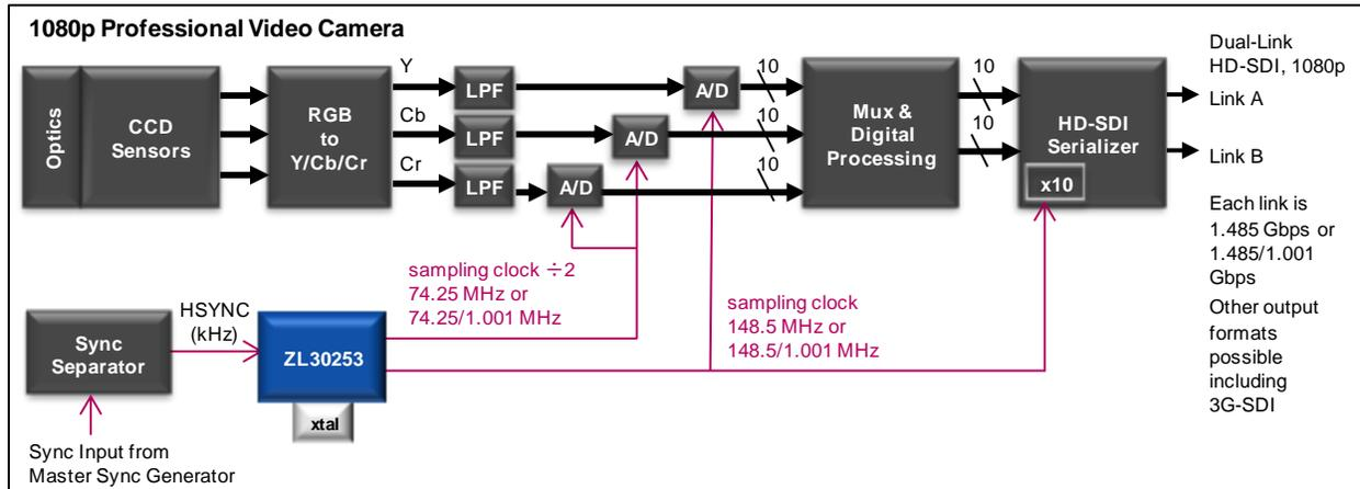
Figure 4 - Frequency Conversion from Low-Frequency Input Clock Using Microsemi's ZL30253
