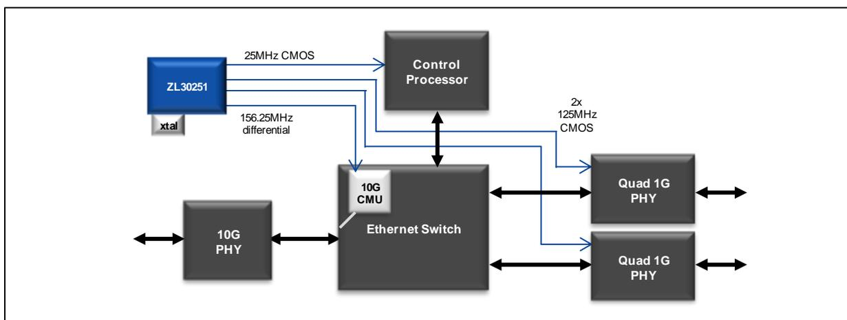
Figure 2 - Clock Synthesis for an Ethernet System Using Microsemi's ZL30251
