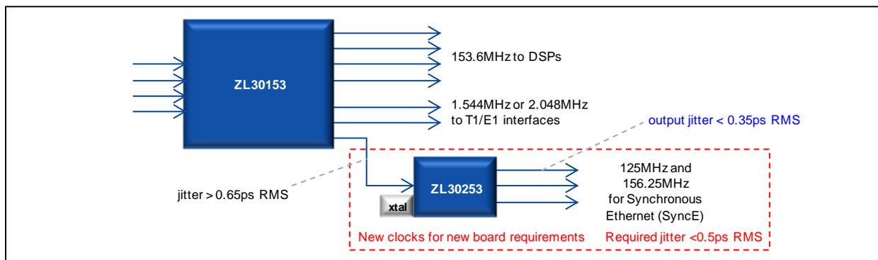
Figure 5 - Add-On Frequency Conversion and Jitter Attenuation Using Microsemi's ZL30253
