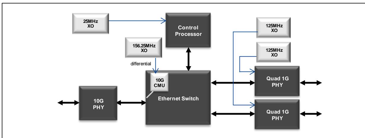
Figure 1 - Clock Synthesis for an Ethernet System Using XOs
