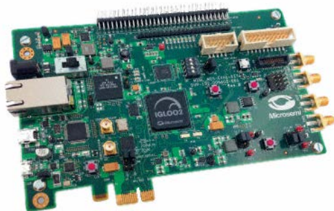
Figure 1: IGLOO2 FPGA Chip with Evaluation Board
