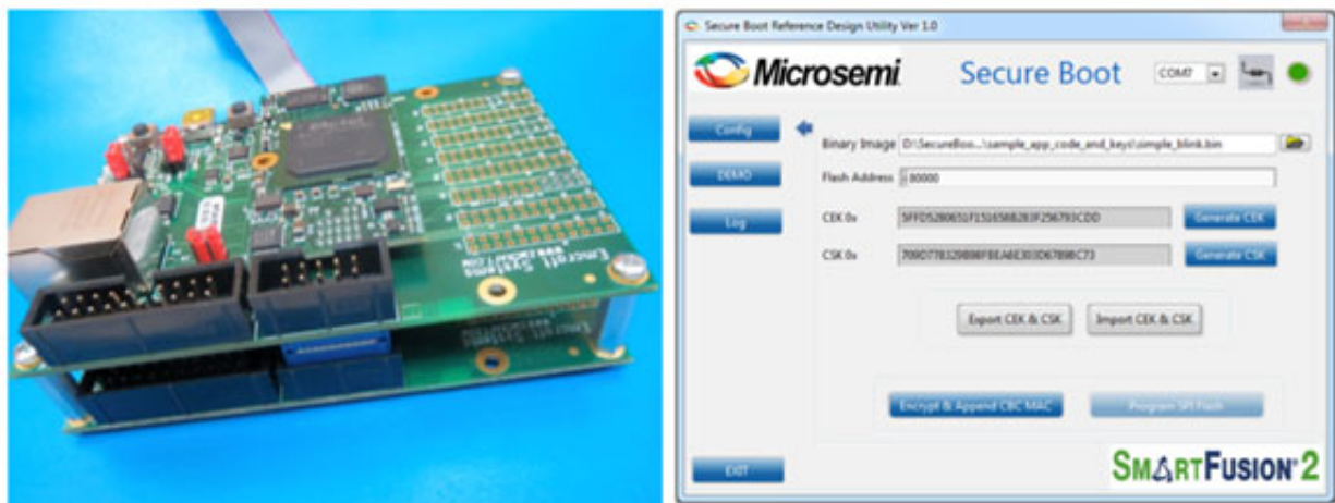
Figure 11: Secure Boot Reference Design Hardware and Configuration Mode Screen
