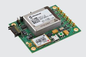
Standard outputs, through a low-noise distribution amplifier, include four 10 MHz sine wave outputs, one 5 MHz CMOS output, and one 1PPS output. Other standard features include—a  $16 \times 2$  character LCD driver (display not included) and a phase noise filter. The unit can be powered from standard aircraft or vehicle power with an 8V to 36V operating range, with a built-in reverse polarity protection. Alternatively the unit can be powered through a 5V mini-USB power supply.
